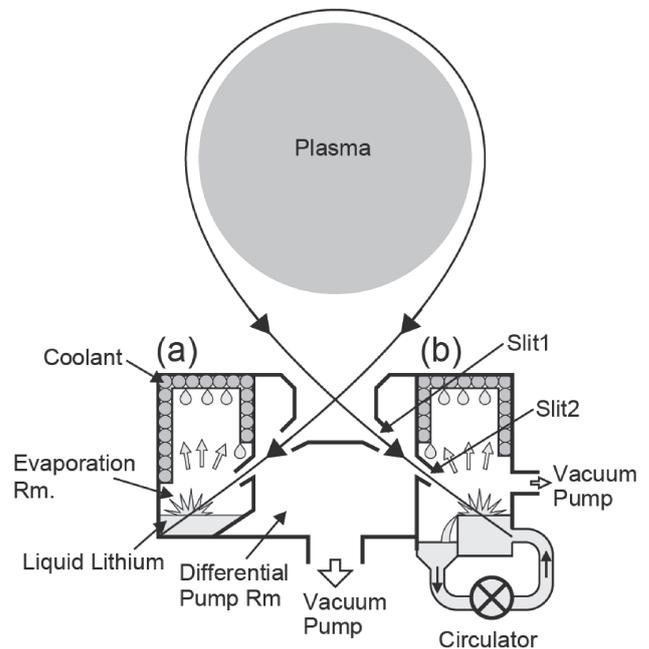
Fig.1 Liquid lithium divertor system. This system works both in tokamak and helical system.
