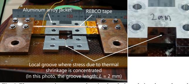
Fig. 4. Element experiment setup that simulate  $I_c$  degradation due to thermal shrinkage
