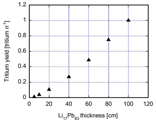
Figure 8. Tritium yield in the Li<sub>17</sub>Pb<sub>83</sub> core from a DT neutron.
