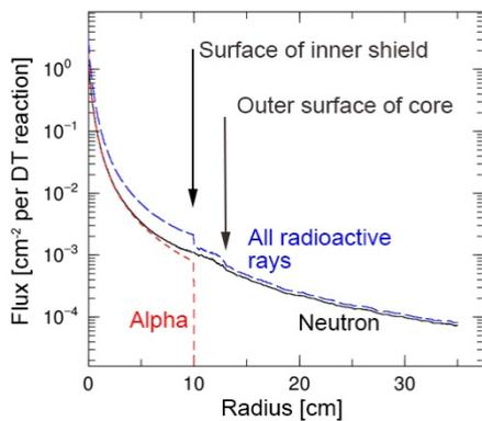
**Figure 3.** Fluxes in the core with the 5 mm B<sub>4</sub>C layer thickness.
