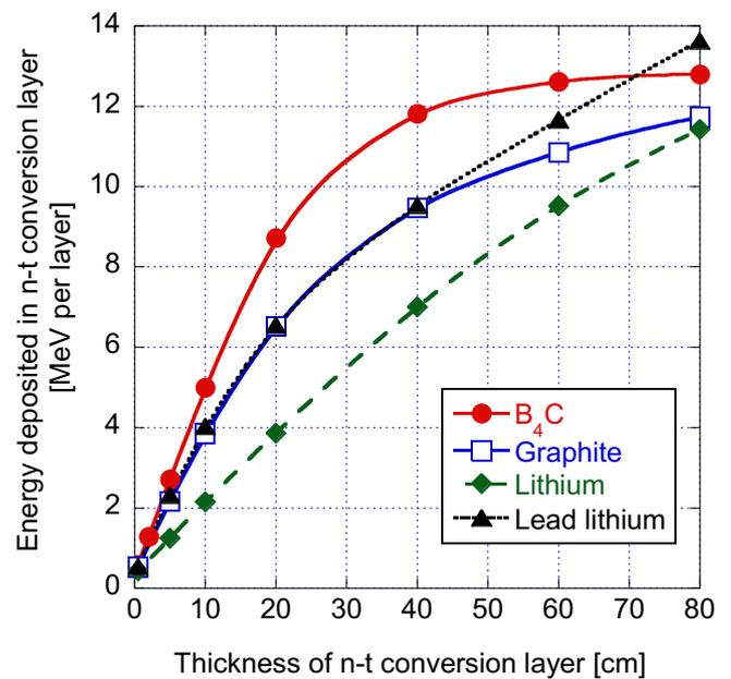
**Figure 4.** Energy deposited in the n-t conversion layers from a DT fusion reaction.
