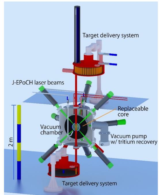
Figure 1. Conceptual drawing of L-Supreme.
