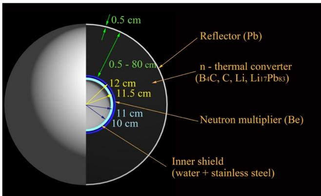
**Figure 2.** Core model for n-t conversion study.
