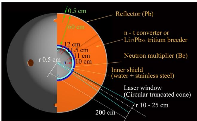
**Figure 9.** Core model with 12 omnidirectional laser windows. Laser windows are defined as circular truncated cones.
