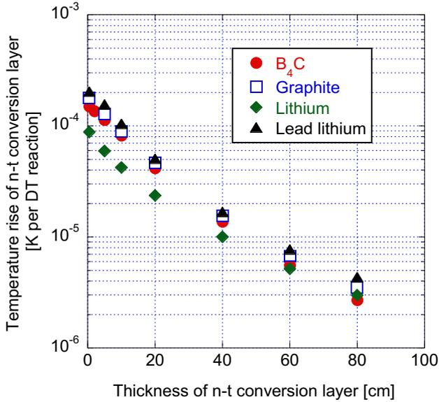
Figure 6. Average temperature rise of n-t conversion layers.
