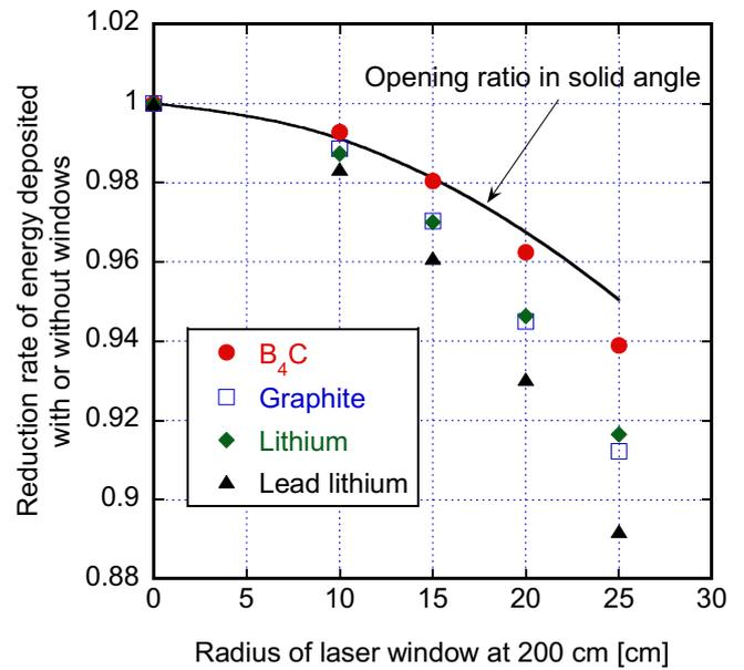
**Figure 10.** Reduction rates of energy deposited.
