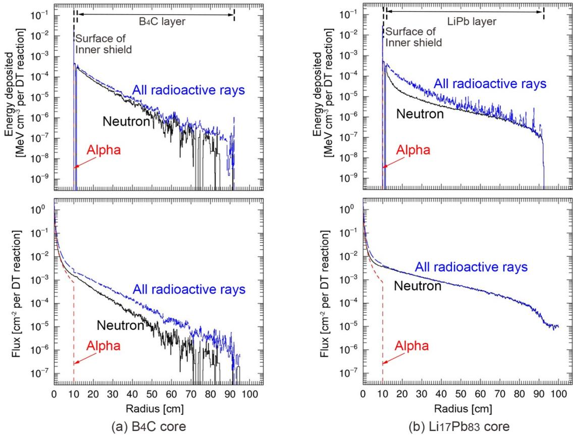
**Figure 5 (a) and (b).** Energy deposited and fluxes in n-t conversion layer from a DT fusion reaction.
