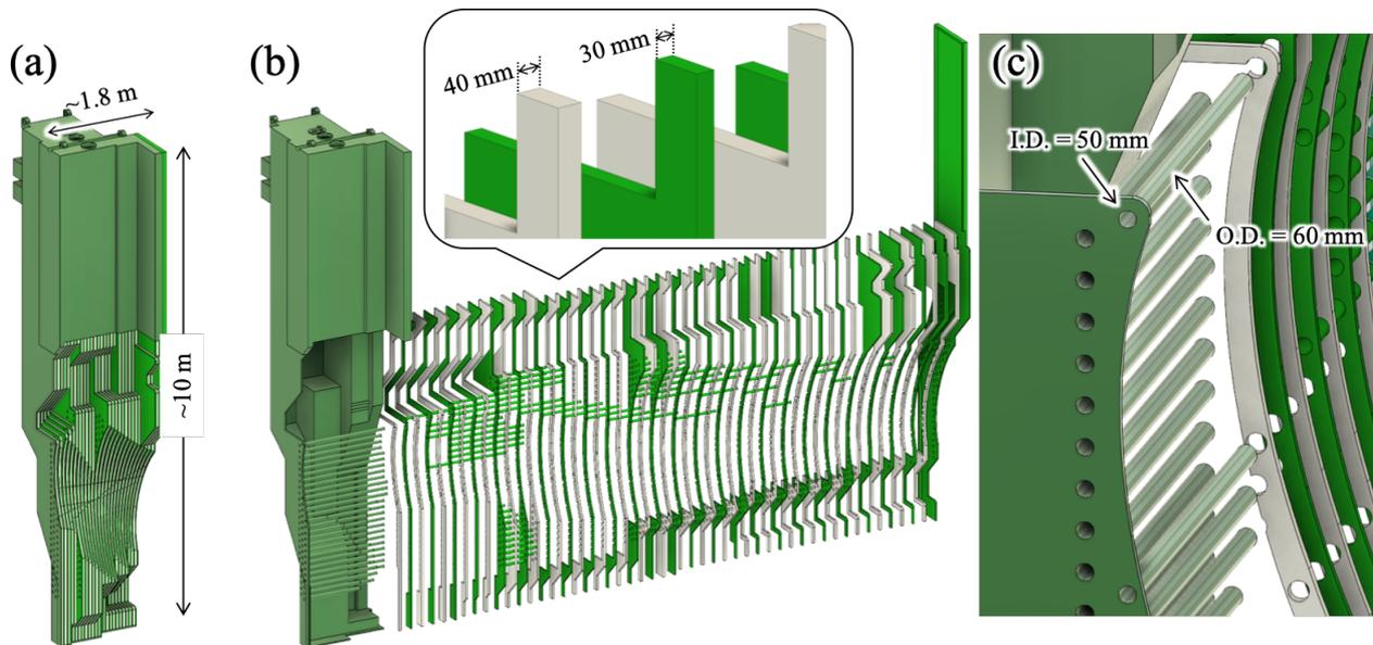
**Figure 3.** (a) Breeding blanket cartridge, BB09, of the CARDISTRY-B3 designed for the FFHR-b3. (b) Exploded view of the BB09. (c) Enlarged view of the horizontal hollow bars.
