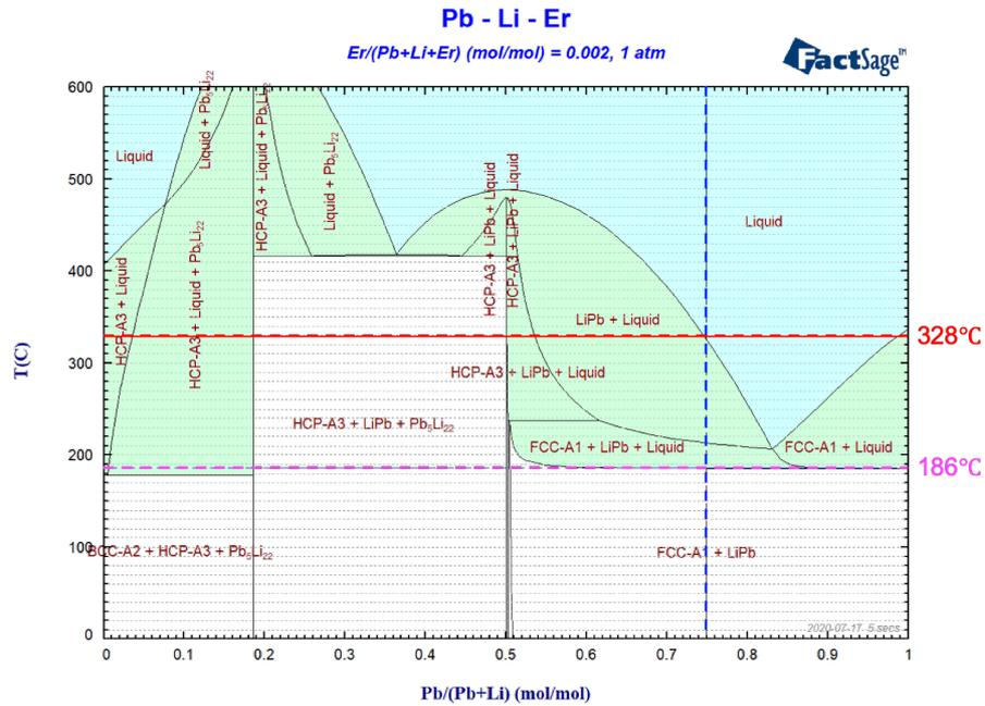
**Figure 15.** Phase diagram of PLE-25. Vertical dashed line denotes PLE-25 ( $\text{Pb}_{74.8}\text{Li}_{25}\text{Er}_{0.2}$ ). Horizontal solid and dashed lines denote the liquid phase temperature and melting point, respectively.
