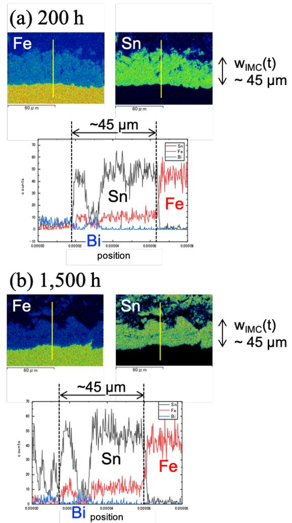
**Figure 24.** Results of the compositional analysis by EDX on the IMC layer formed on the outer periphery of the sample pipe immersed in SBLE-25 at  $400^\circ\text{C}$  for (a) 200 h, and (b) 1,500 h, respectively.
