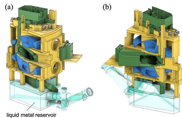
**Figure 6.** Bird's eye views of one toroidal section of the CARDISTRY-B3.
