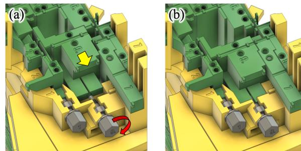
**Figure 7.** (a) Before and (b) after the sliding action of the BB09 by the bolt mechanism.
