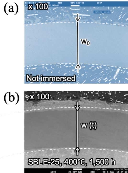
**Figure 23.** SEM images of the sample pipe sliced at (a) a part not immersed in SBLE-25, and (b) a part immersed in SBLE-25 at 400°C for 1,500 hours. White broken curves denote the initial positions of outer and inner edges of the sample pipe.
