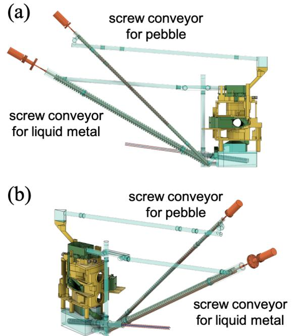
**Figure 10.** (a) A side view and (b) a bird's eye view of the screw conveyors for pebble and liquid metal.
