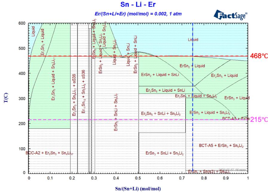
**Figure 17.** Phase diagram of SLE-25. Vertical dashed line denotes SLE-25 ( $\text{Sn}_{74.8}\text{Li}_{25}\text{Er}_{0.2}$ ). Horizontal solid and dashed lines denote the liquid phase temperature and melting point, respectively.
