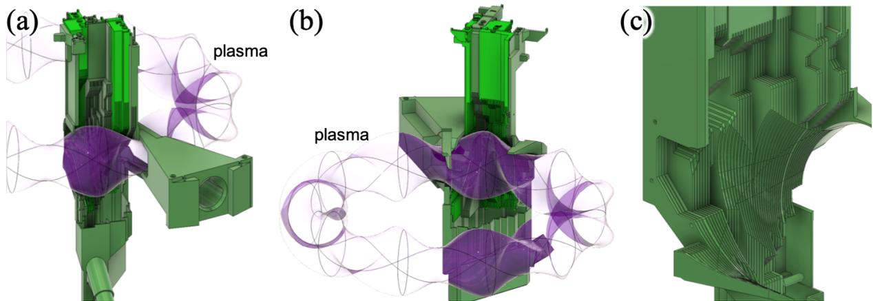
**Figure 2.** Schematic views of the breeding blanket cartridges of the CARDISTRY-B3 on (a) the inboard side and (b) the outboard side of the torus. (c) An enlarged view of the breeding blanket cartridges on the outboard side.
