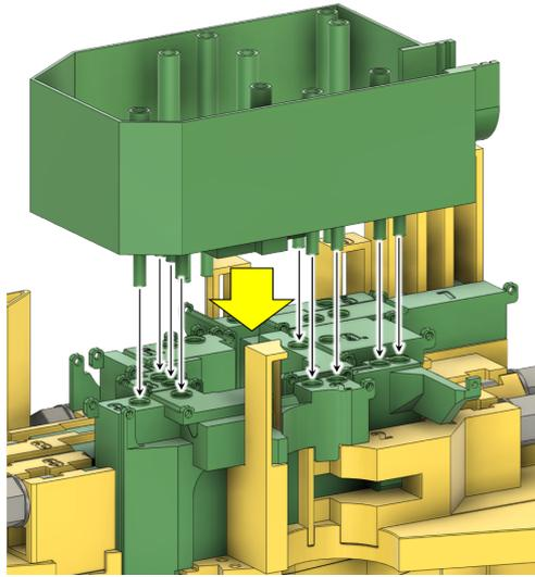
**Figure 8.** Installation of BB10. Injection tubes for liquid metal supply are inserted to the holes of the cartridges.
