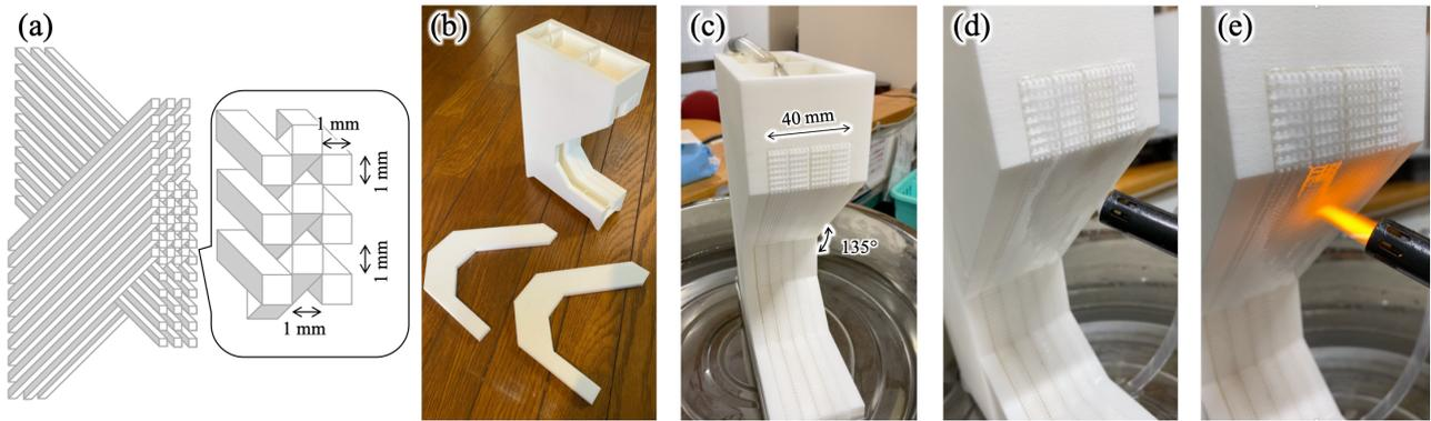
**Figure 4.** (a) Design of a porous material for 3D printing. (b) 3D printed porous plates. (c) A test device consisted of four porous plates. (d) Porous plates covered with the surface flow of water oozed from inside of the test device. (e) Fire resistance test of the porous plates covered by water surface flow.
