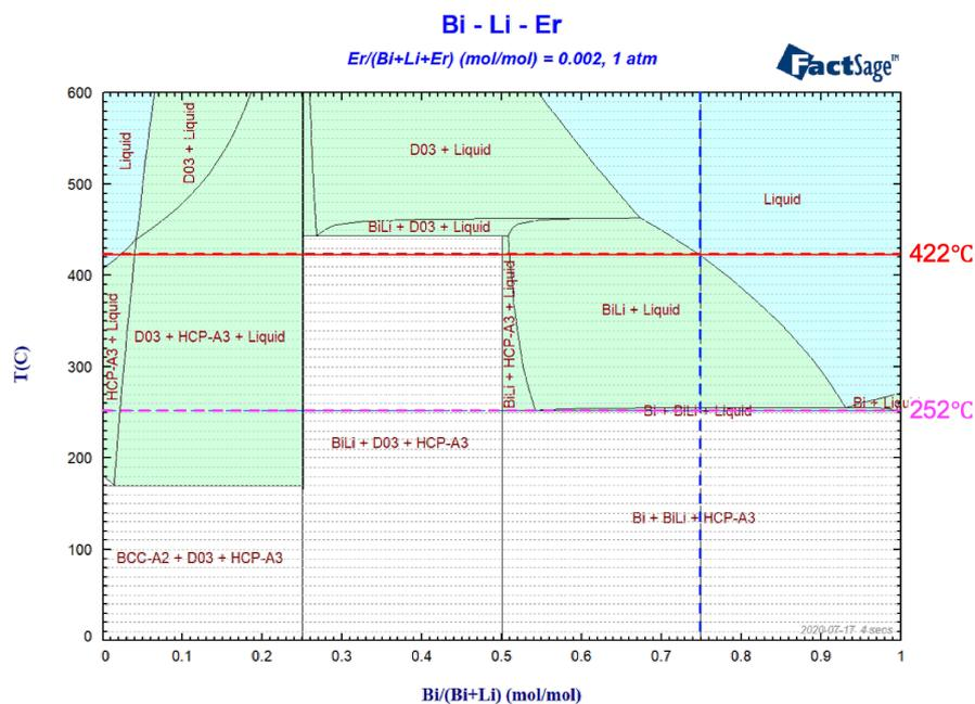
**Figure 16.** Phase diagram of BLE-25. Vertical dashed line denotes BLE-25 ( $\text{Bi}_{74.8}\text{Li}_{25}\text{Er}_{0.2}$ ). Horizontal solid and dashed lines denote the liquid phase temperature and melting point, respectively.
