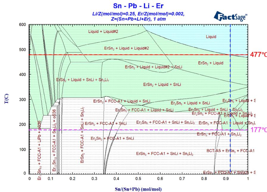
**Figure 18.** Phase diagram of SLPE-25. Vertical dashed line denotes SLPE-25 ( $\text{Sn}_{68.8}\text{Li}_{25}\text{Pb}_6\text{Er}_{0.2}$ ). Horizontal solid and dashed lines denote the liquid phase temperature and melting point, respectively.
