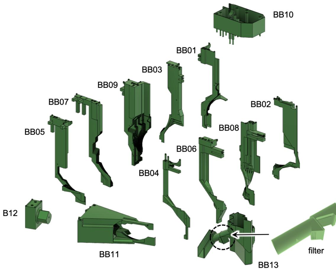
**Figure 5.** An exploded view of breeding blanket cartridges in a 1/10 toroidal section of the CARDISTRY-B3.
