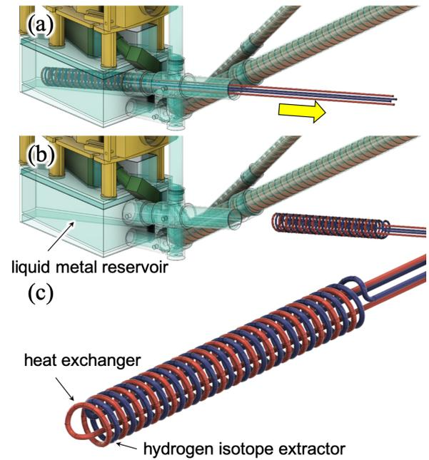
**Figure 12.** (a) Arrangement of the heat exchanger and hydrogen isotope extractor, (b) after being taken out for maintenance, and (c) a close-up view of it.
