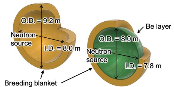
**Figure 14.** Spherical models with or without the Be neutron multiplier layer.
