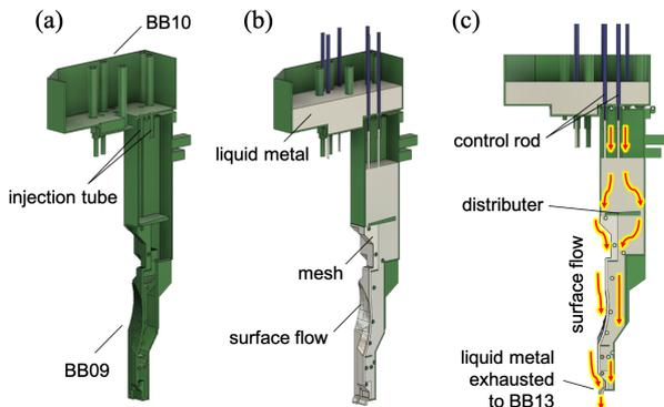
**Figure 9.** Sliced views of BB09 and BB10 (a) without liquid metal and (2) with liquid metal. (c) A side view of BB09 and BB10 with liquid metal. The arrows in (c) denote the liquid metal flow inside and the surface of the BB09.
