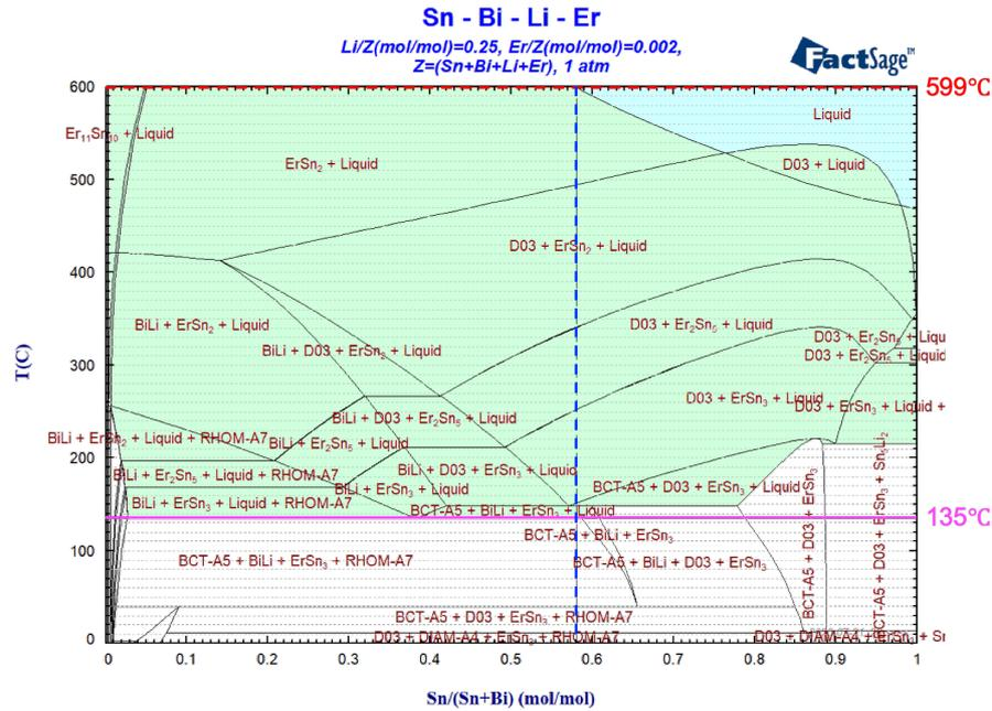
**Figure 19.** Phase diagram of SBLE-25. Vertical dashed line denotes SBLE-25 ( $\text{Sn}_{43.3}\text{Bi}_{31.5}\text{Li}_{25}\text{Er}_{0.2}$ ). Horizontal solid and dashed lines denote the liquid phase temperature and melting point, respectively.
