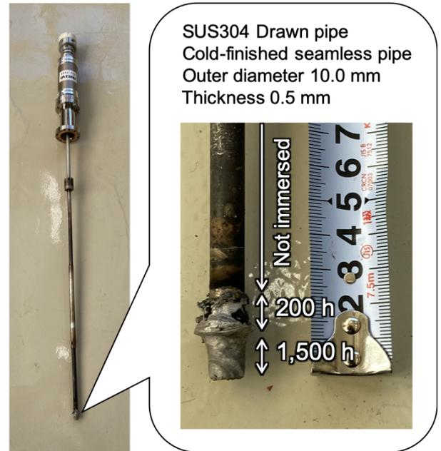
Figure 22. Overall photo and enlarged photo of the sample pipe of SUS304.
