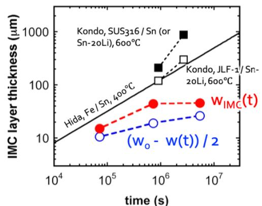
**Figure 25.** Time trend of the IMC layer thickness,  $w_{\text{IMC}}(t)$ , and the corrosion layer thickness defined by  $(w_0 - w(t)) / 2$ , together with the former experimental results given by Hida [31] and Kondo [32].
