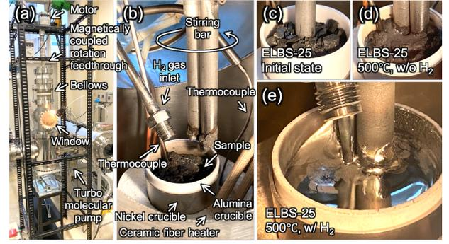
**Figure 20.** (a) A vacuum device used for basic experiment of FLM. (b) Internal view of the experimental device. (c) SBLE-25 in its initial state. (d) SBLE-25 heated up to  $500^\circ\text{C}$  without hydrogen gas puffing. (e) SBLE-25 heated up to  $500^\circ\text{C}$  with hydrogen gas puffing.
