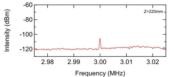
(a) Spectrum of ICRF wave measured by the EO sensor
