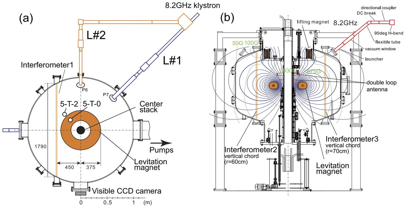
FIG. 4. Magnetosphere plasma device RT-1. (a) Top view and (b) cross sectional view. For the electric field measurements, the EO sensor head was inserted from the 5-T-0 ( $R = 0.245$  m) and 5-T-2 ( $R = 0.72$  m) ports. The double-loop antenna for ICRF heating is mounted on the center stack.
