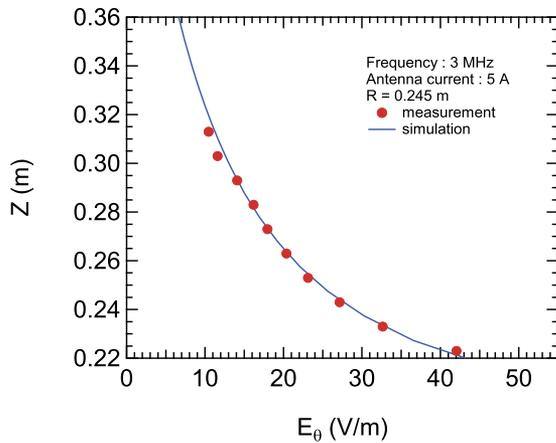
FIG. 7. Electric field profile of  $E_0$  at 3 MHz measured by the EO sensor (closed circles) in RT-1 in the air experiments. The simulation result (blue curve) is also plotted.
