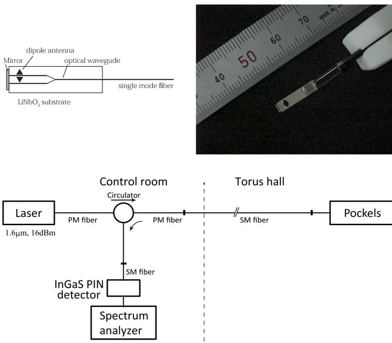
FIG. 1. Measurement setup of electric field with the EO sensor. Upper left shows the internal structure of the EO sensor tip. Upper right is a photograph of the EO sensor. The acrylic resin case, which normally protects the tip from shock, has been dismantled for the photograph.
