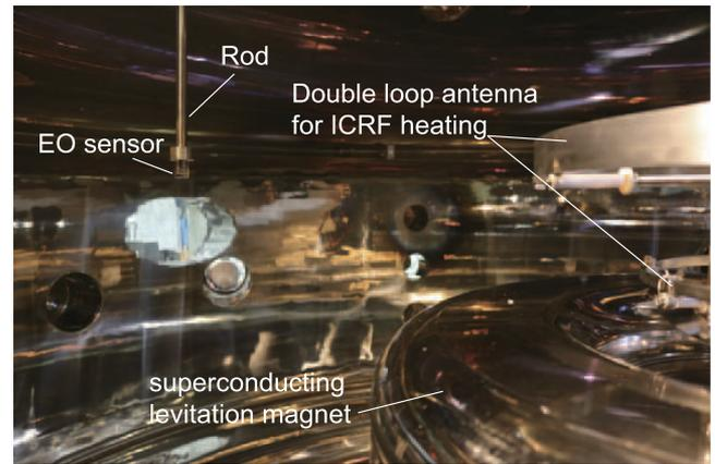
FIG. 8. The EO sensor mounted inside the supporting rod is inserted from the top port. The vacuum vessel of RT-1 contains the levitation superconducting magnet and the double-loop antenna for ICRF heating.
