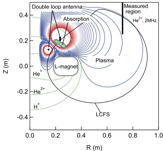
FIG. 9. Contours of the electric field  $E_\theta$  excited by the double-loop antenna in helium plasma. L-magnet indicates the levitation magnet. The antennas are located outside the LCFS. The contours of the power absorption area for  $\text{He}^{2+}$  are also plotted. The ion cyclotron layers for  $\text{H}^+$ ,  $\text{He}^{2+}$ , and  $\text{He}^+$  are depicted.
