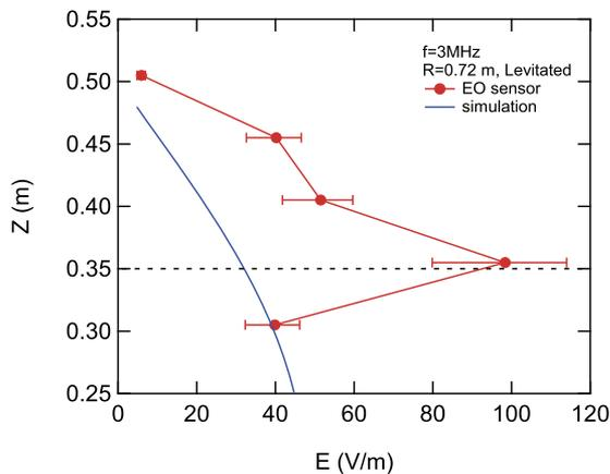
FIG. 10.  $E_\theta$  (closed circles) vertically measured by the EO sensor along  $R = 0.72$  m in helium plasma. The ICRF power is 7 kW. The separatrix (dashed line) is located at  $(R, Z) = (0.72$  m, 0.35 m). The input parameter for the simulation was the measured antenna current (252 A).
