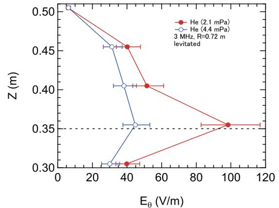
FIG. 11.  $E_\theta$  measured by the EO sensor in helium plasmas. The helium gas pressures were 2.1 mPa (closed circles) and 4.4 mPa (open circles).
