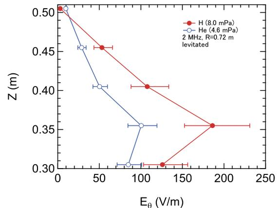
FIG. 12.  $E_\theta$  measured by the EO sensor in plasmas. The fill gas pressures are mixed hydrogen at 8.0 mPa and helium at 0.6 mPa (closed circles) and helium at 4.6 mPa (open circles).
