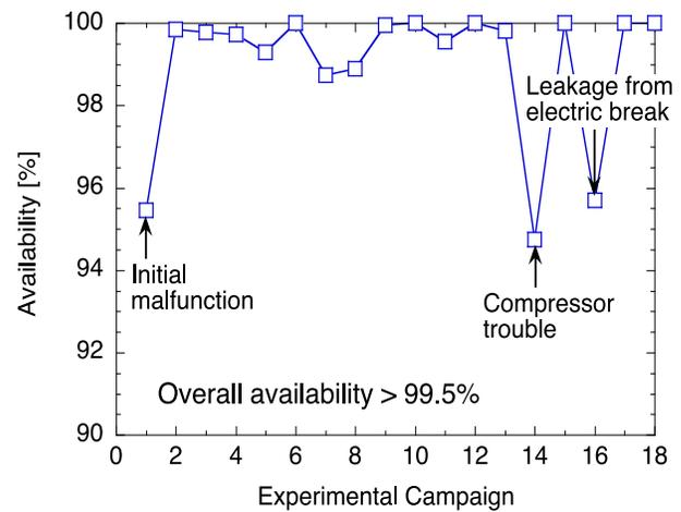
Figure 2 Availability of the LHD cryogenic system.
