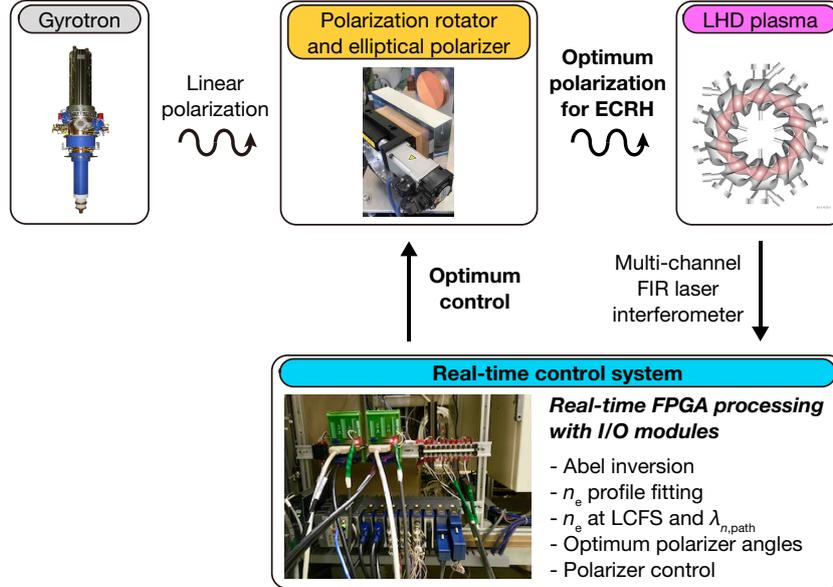
Figure 2: Schematic real-time control system of the incident EC wave polarization.
