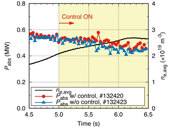
Figure 7: Time evolution of absorbed power of the 5.5-U 77 GHz EC wave during density ramp-up to  $\sim 3 \times 10^{19} \text{ m}^{-3}$  in the cases with and without the polarizer motion control from  $t = 5$  s.
