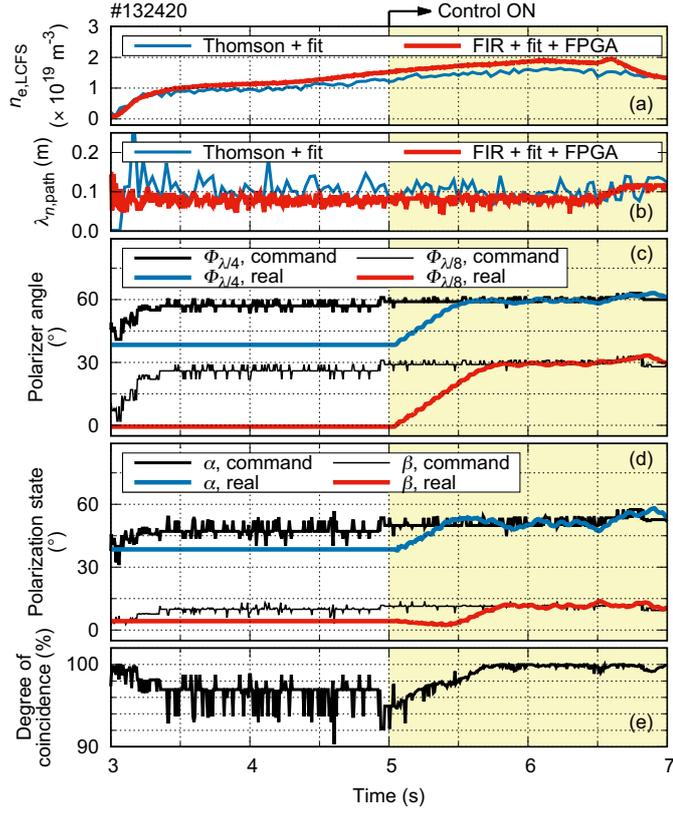
Figure 5: Typical result of polarization optimization control: Lines are plotted as in Fig. 4. The polarizer motion control was conducted from  $t = 5$  s.
