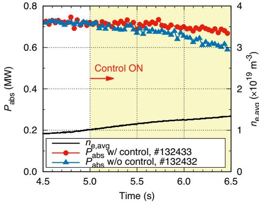
Figure 6: Time evolution of absorbed power of the 5.5-U 77 GHz EC wave for relatively low-density plasma of line-averaged electron density of  $\sim 1 \times 10^{19} \text{ m}^{-3}$  in the cases with and without the polarizer motion control from  $t = 5$  s.
