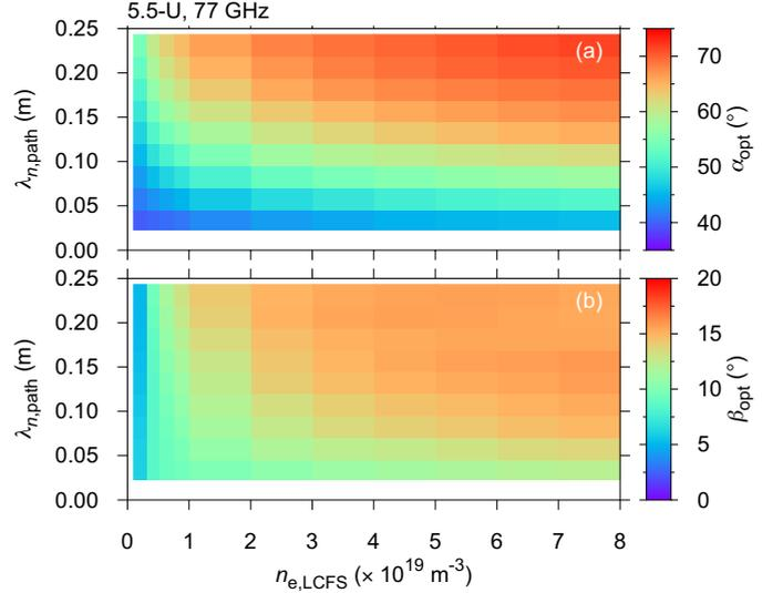
Figure 1: Dependence of optimum incident EC wave polarization on peripheral electron density profile: (a) the optimum polarization rotation angle  $\alpha_{opt}$  and (b) the optimum polarization ellipticity  $\beta_{opt}$  for different electron density  $n_{e,LCFS}$  at the LCFS and the scale length for the density gradients  $\lambda_{n,path}$  along the EC beam path.
