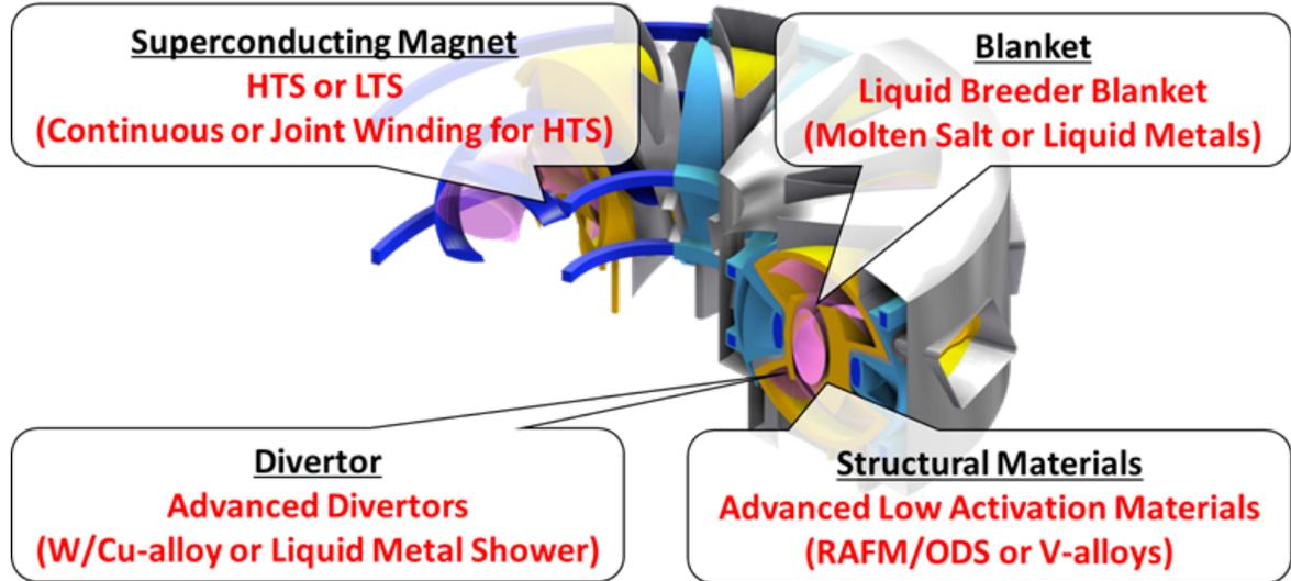
Fig.2 Some options being considered in the design of FFHR-d1<sup>12</sup>.
