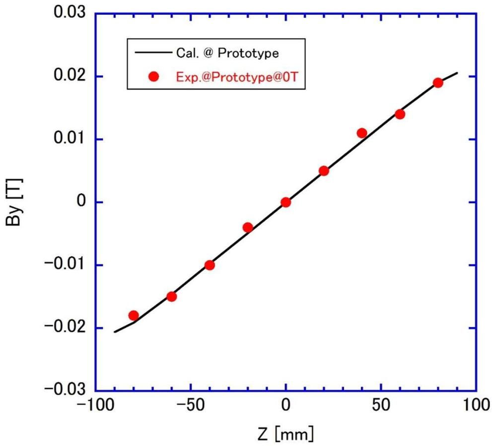
Fig. 35 Measured and calculated self-field of the prototype joint.  $z = 0$  mm is the center of the prototype joint in the longitudinal direction. The position of the Hall sensors is 0 mm in the x direction.
