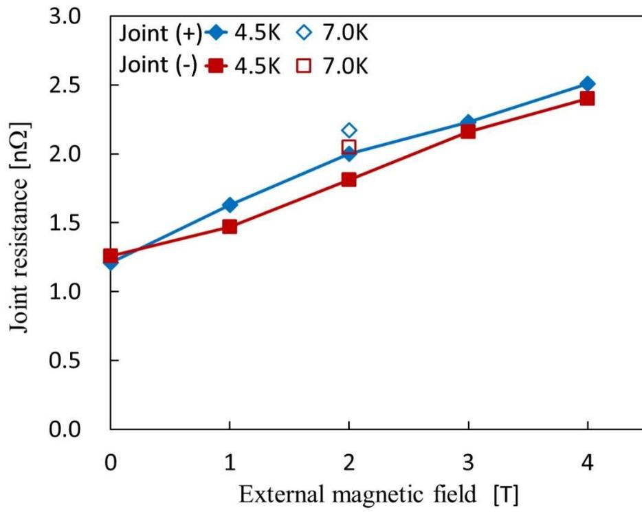
Fig. 44 Joint resistances of the pancake joint for the CS coil.
