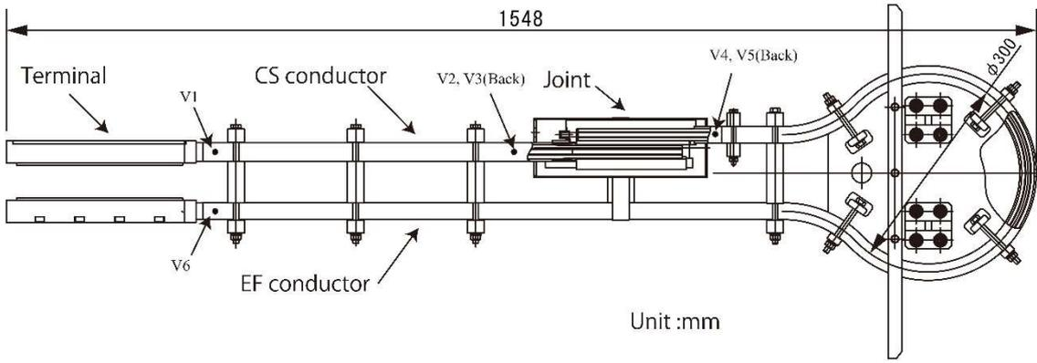
Fig. 41 Schematic view of the terminal joint sample for the CS coil.
