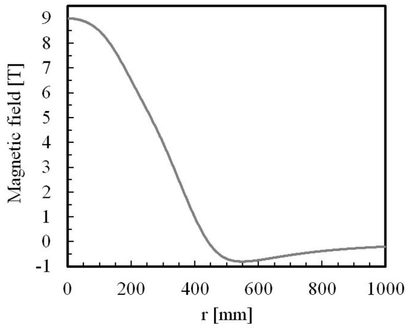
Fig. 2 Magnetic field distribution of the split coil in the test facility for large superconductors. Sign  $r$  is the radial distance from the center of the split coil in the test facility.
