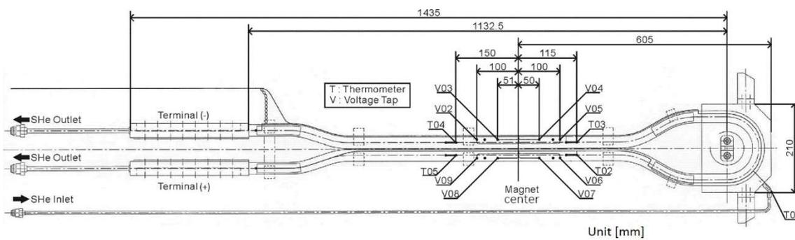
Fig. 23 Schematic view of the CS conductor sample.
