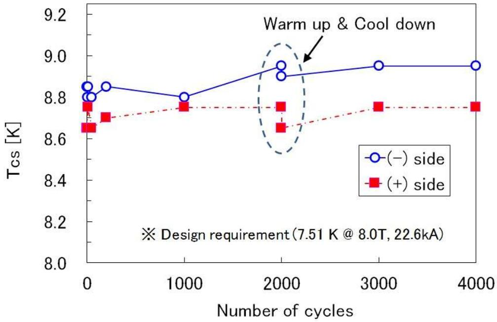
Fig. 26  $T_{cs}$  measurement results of the CS conductor sample under the EM and thermal cycles.
