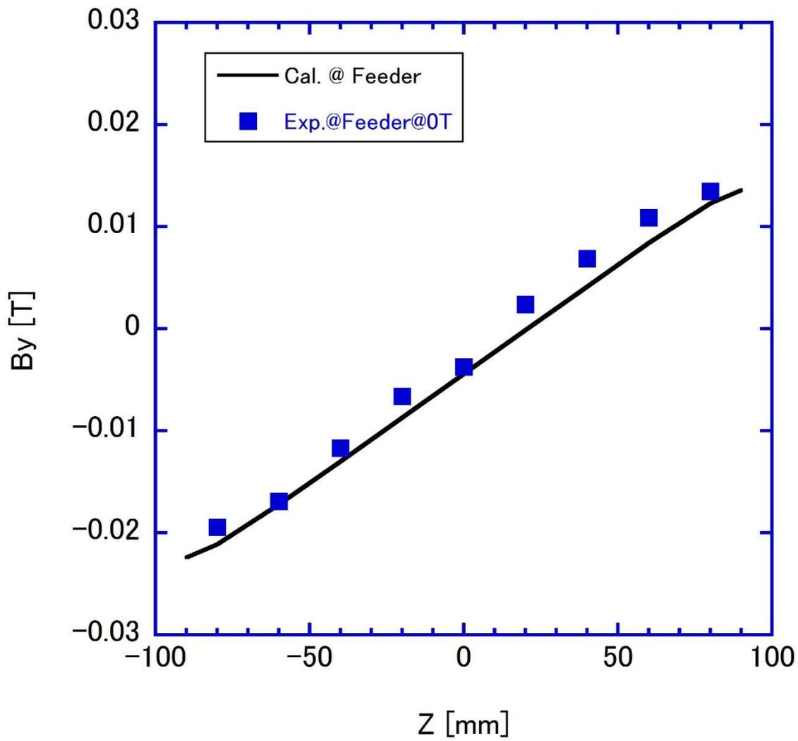
Fig. 36 Measured and calculated self-field of the feeder joint.  $z = 0$  mm is the center of the prototype joint in the longitudinal direction. The position of the Hall sensors is 5 mm in the x direction.
