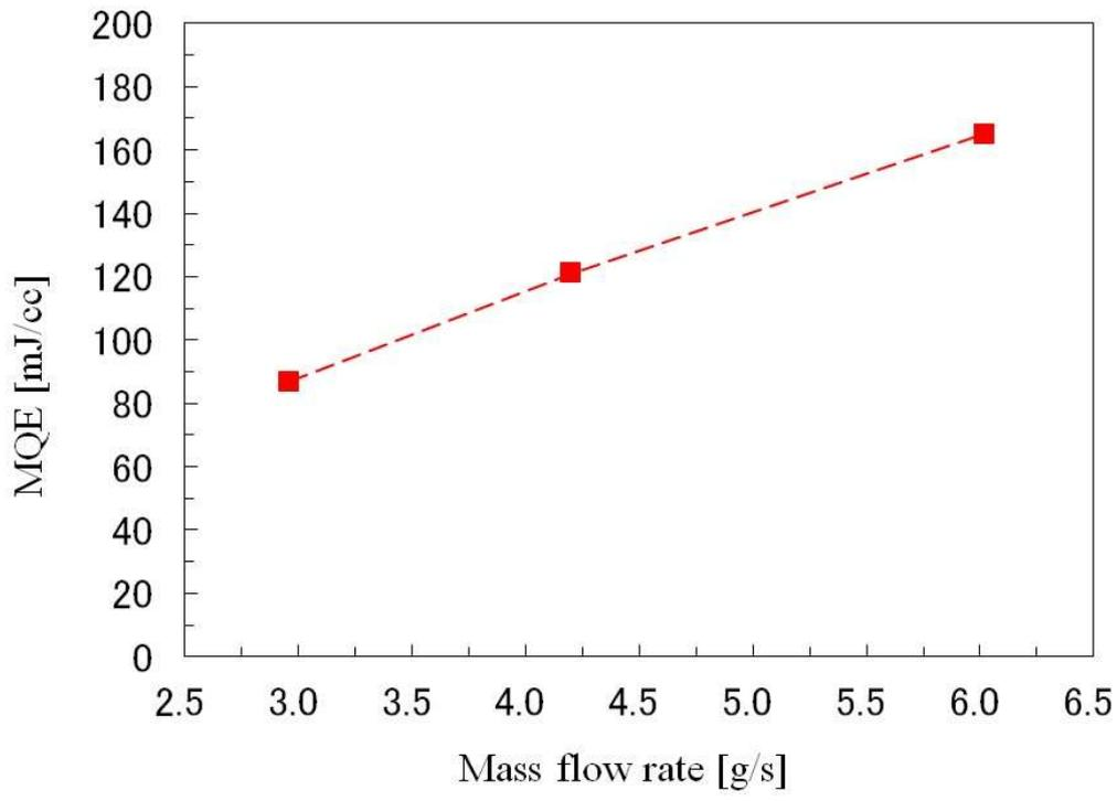
Fig. 17 Stability test results of the EF-L conductor sample for each mass flow rate.
