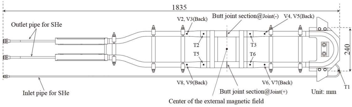
Fig. 37 Schematic view of the pancake joint sample for the CS coil.
