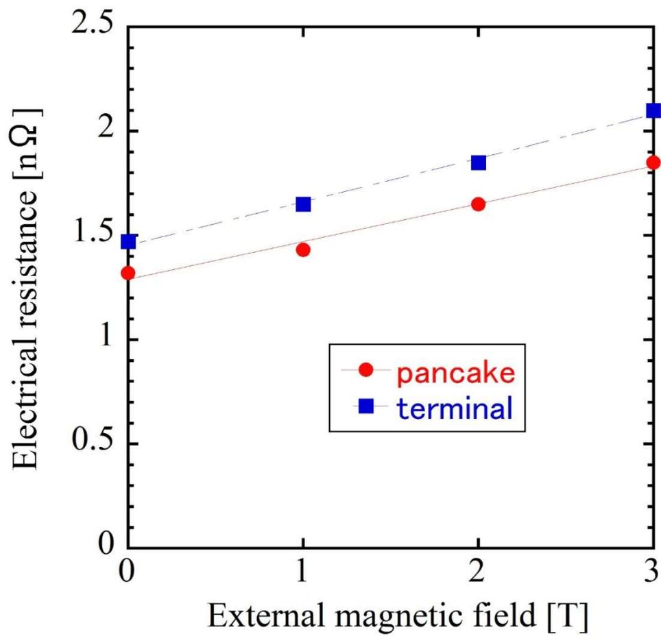
Fig. 33 Joint resistances of the pancake and terminal joints.
