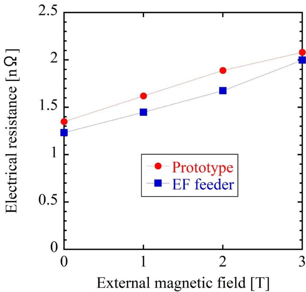
Fig. 34 Joint resistances of the prototype and feeder joints for the EF coil.
