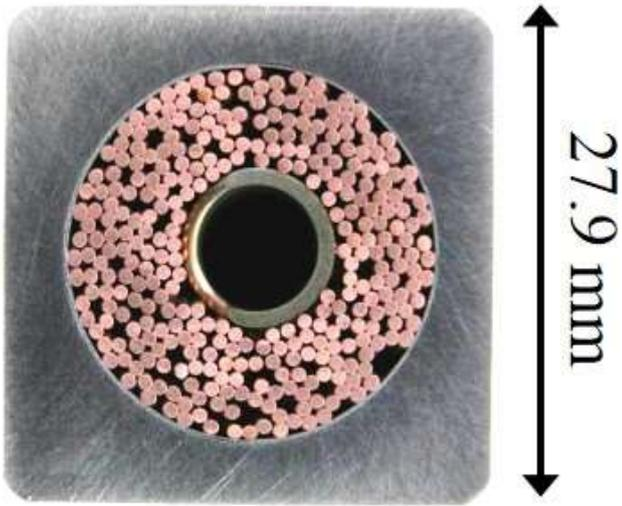
Fig. 22 Cross-section of the CS conductor.
