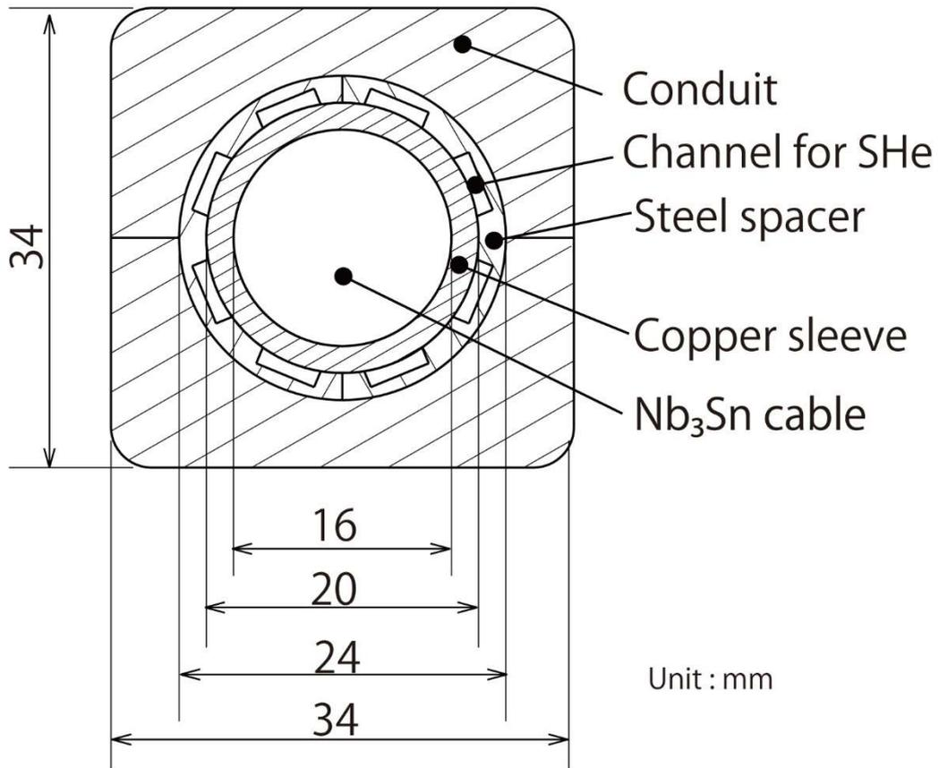
Fig. 40 Cross-section of the butt joint.
