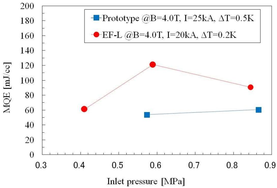
Fig. 18 Stability test results of the prototype and EF-L conductor samples for each inlet pressure.
