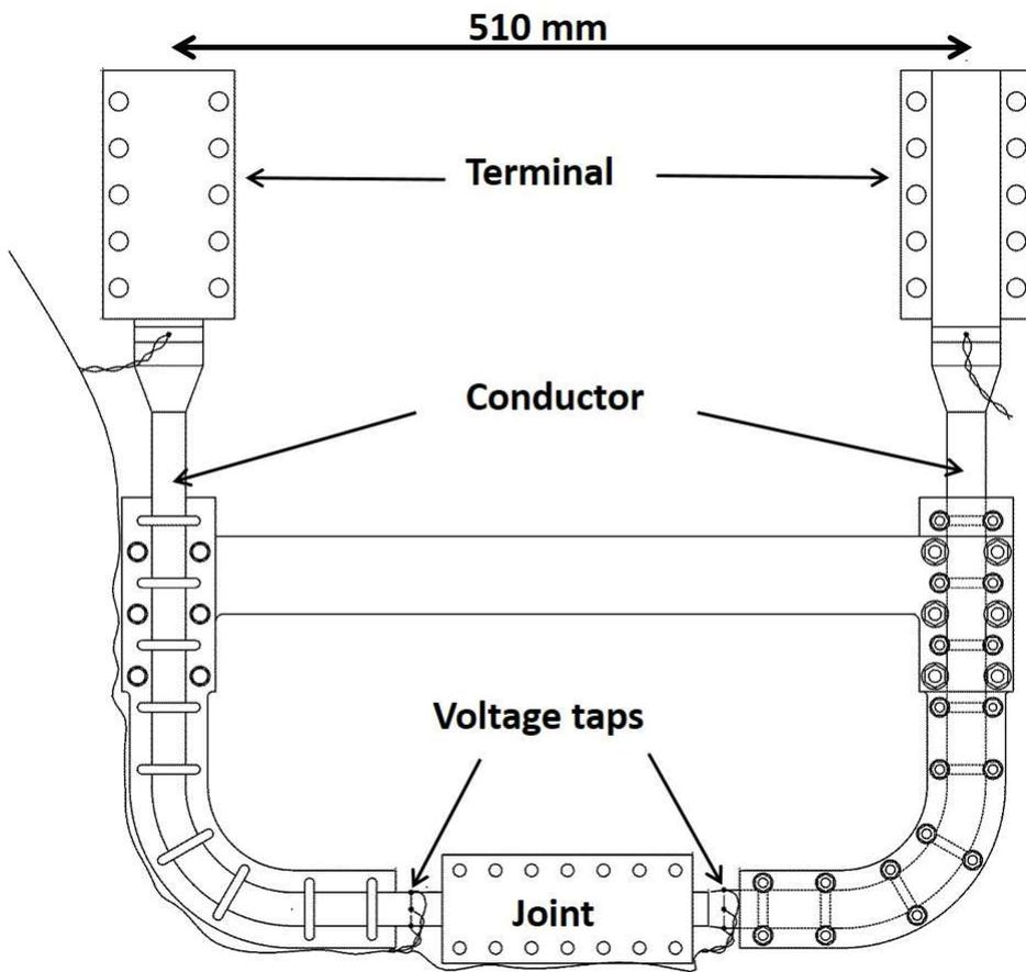
Fig. 27 Schematic view of the prototype joint sample.
