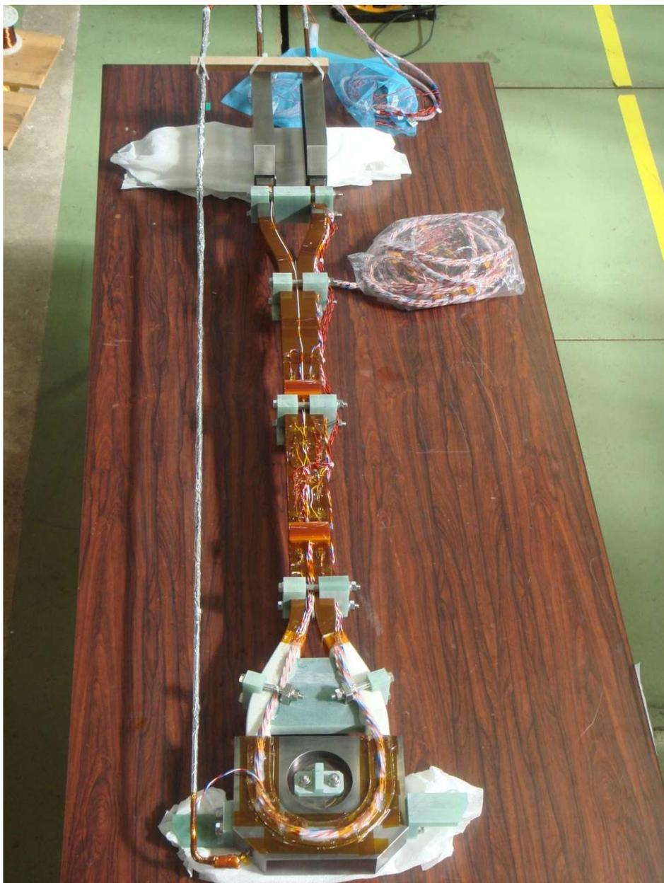
Fig. 24 Photograph of the CS conductor sample.
