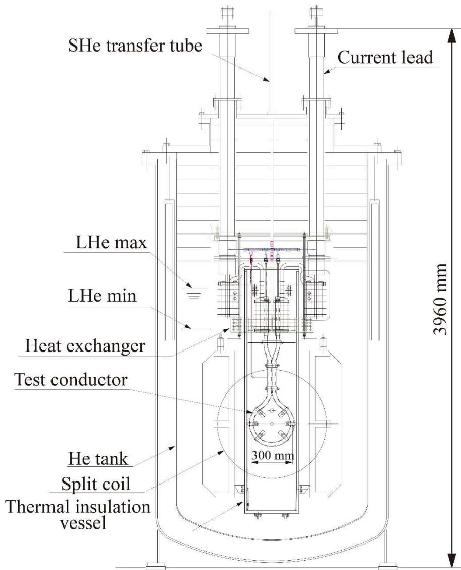
Fig. 3 Schematic view of the test facility for large superconductors.
