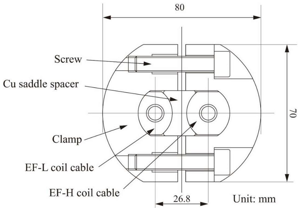
Fig. 32 Cross-section of the pancake joint for the EF coil.
