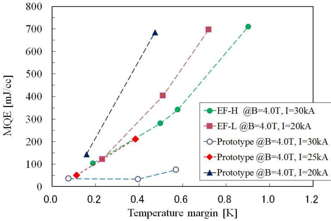
Fig. 16 Stability test results of the EF conductor sample for each temperature margin.
