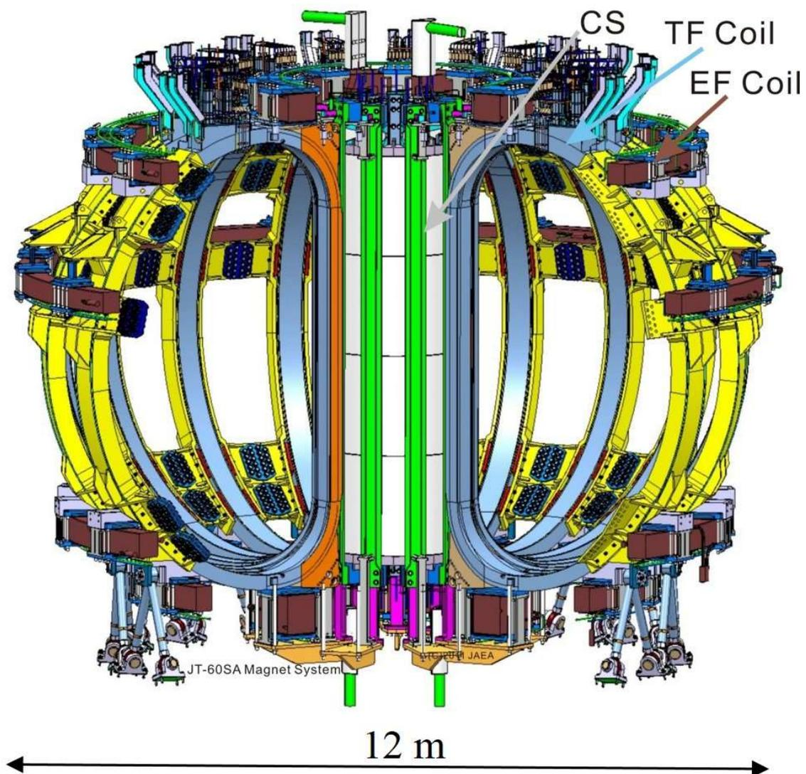
Fig. 1 Schematic view of the JT-60SA magnet system.
