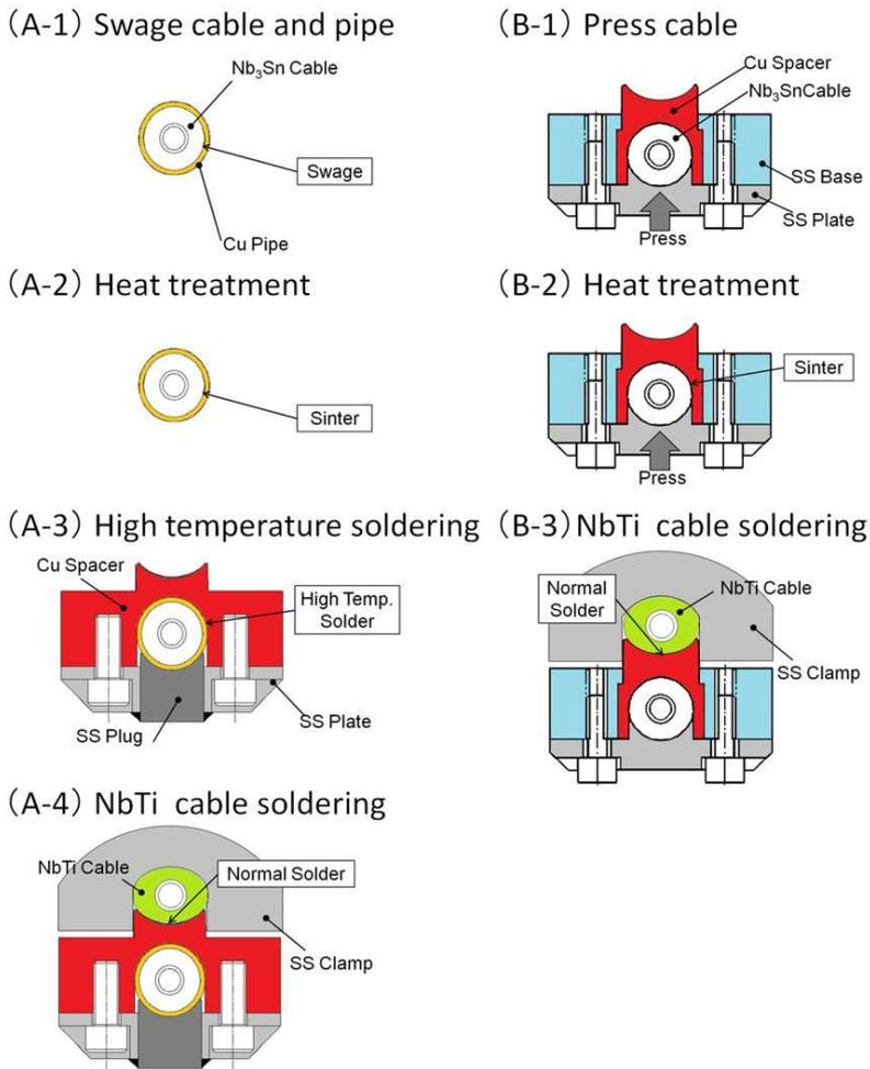
Fig. 43 Fabrication process of the “Type A” and “Type B” joint for the terminal joints.
