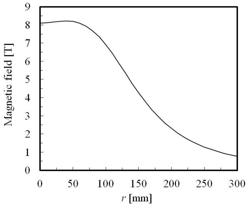
Fig. 6 Magnetic field distribution of the split coil in the test facility for middle-sized superconductors. Sign  $r$  is the radial distance from the center of the split coil in the test facility.
