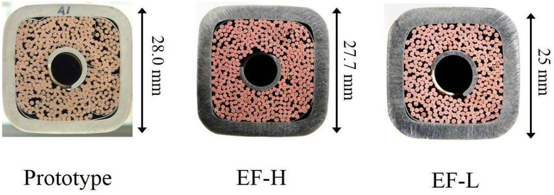
Fig. 7 Cross-sections of the EF coil conductors.
