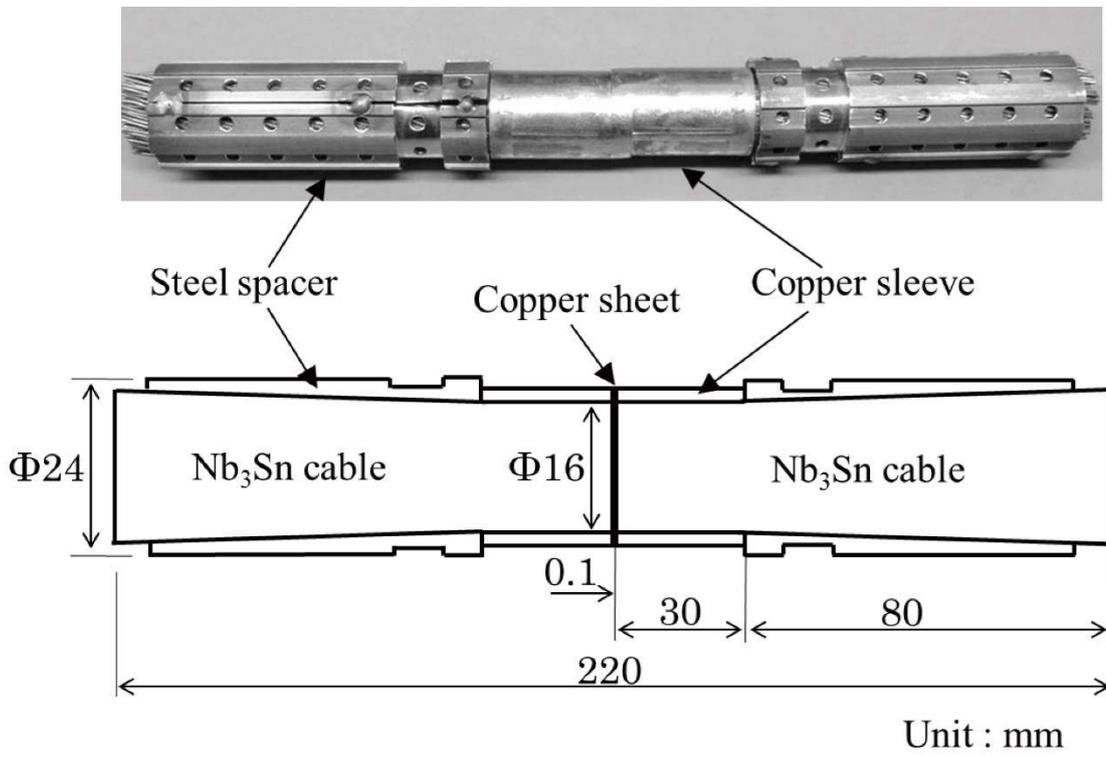
Fig. 39 Configuration and photograph of the butt joint.
