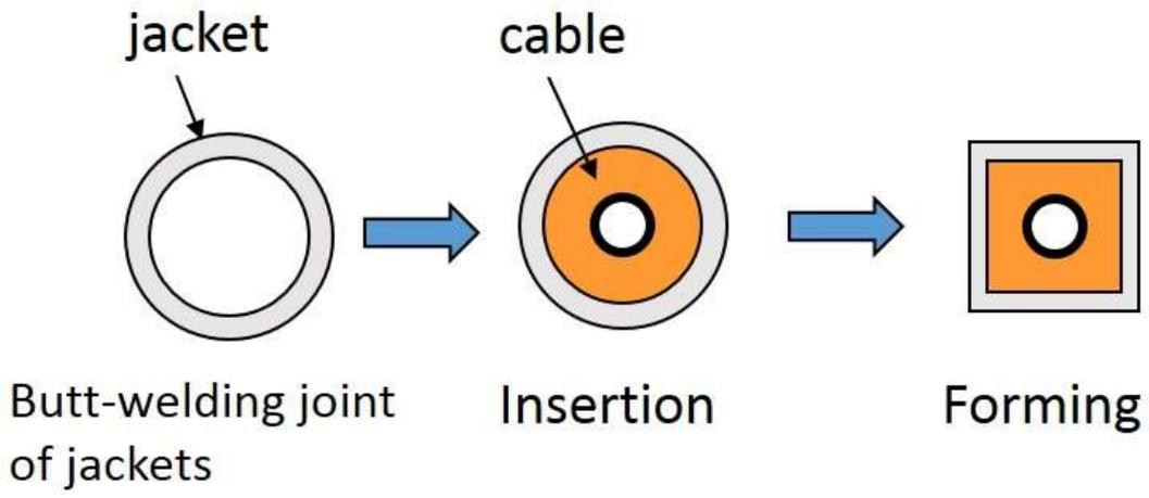
Fig. 8 Fabrication process of the EF coil conductor.
