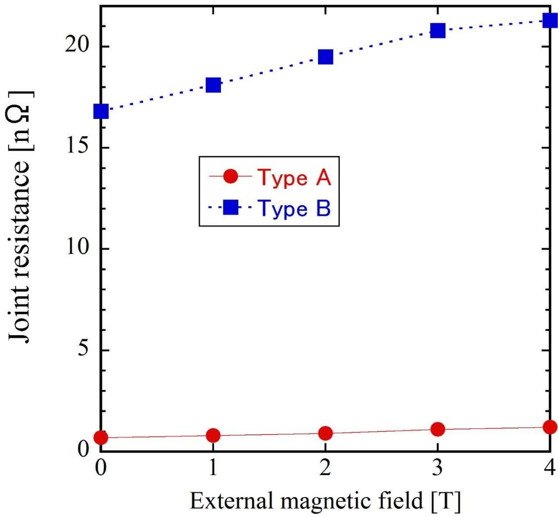
Fig. 45 Joint resistances of the terminal joints for the CS coil.
