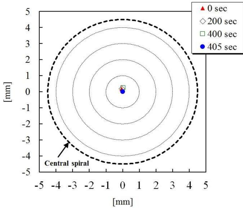
Fig. 20 The position of current center in the cross-section of the EF-L conductor sample during the Tcs measurement. Signs  $\triangle$ ,  $\diamond$ , and  $\square$  show the position of the current center at 0 sec, 200 sec, and 400 sec. Sign  $\bullet$  shows the position of the current center at 405 sec when the normal propagation occurred.
