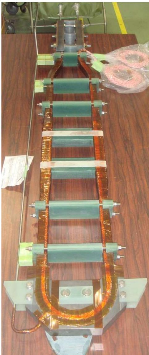
Fig. 38 Photograph of the pancake joint sample for the CS coil.
