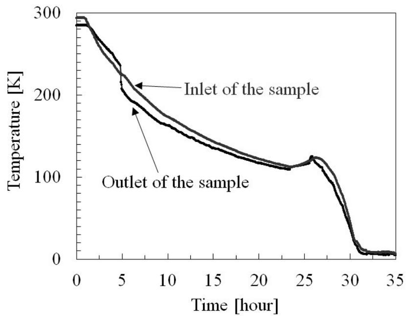
Fig. 4 Cooling curves of a CIC conductor sample in the test facility for large superconductors.
