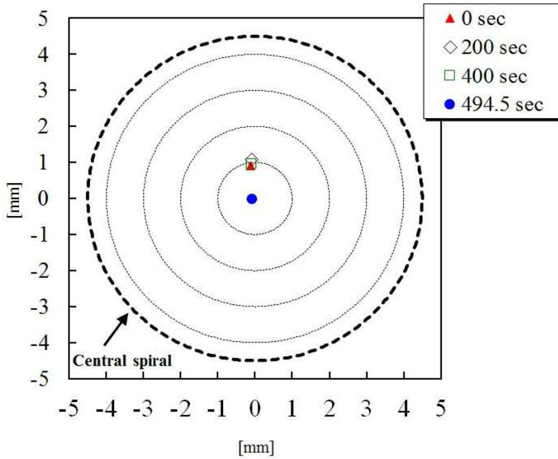
Fig. 21 The position of current center in the cross-section of the prototype conductor sample during the Tcs measurement. Signs  $\triangle$ ,  $\diamond$ , and  $\square$  show the position of the current center at 0 sec, 200 sec, and 400 sec. Sign  $\bullet$  shows the position of the current center at 494.5 sec when the normal propagation occurred.
