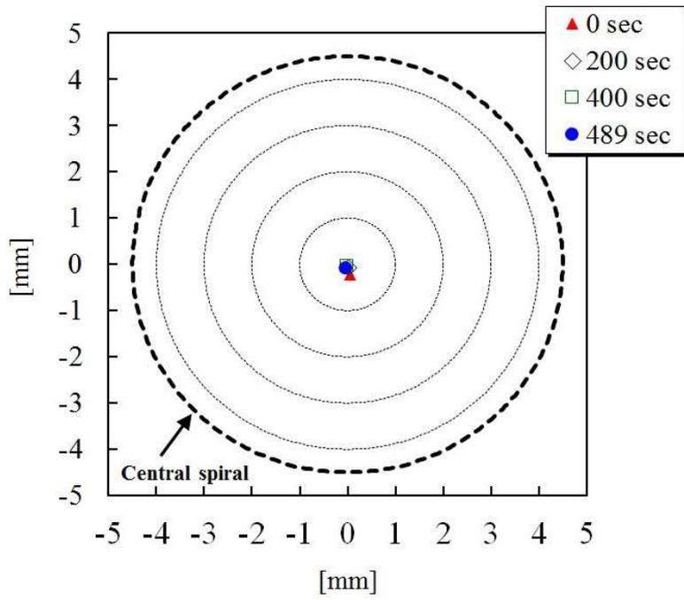
Fig. 19 The position of current center in the cross-section of the EF-H conductor sample during the Tcs measurement. Signs  $\triangle$ ,  $\diamond$ , and  $\square$  show the position of the current center at 0 sec, 200 sec, and 400 sec. Sign  $\bullet$  shows the position of the current center at 489 sec when the normal propagation occurred.
