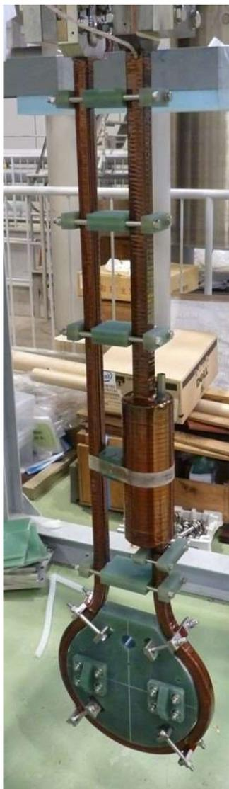
Fig. 42 Photograph of the terminal joint sample for the CS coil.
