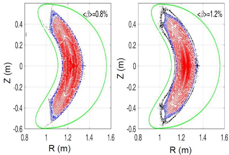
Figure 3. Finite beta MHD equilibrium taking the neoclassical bootstrap current into account. Left:  $\langle\beta\rangle$  of 0.8 %. Right:  $\langle\beta\rangle$  of 1.2 %.
