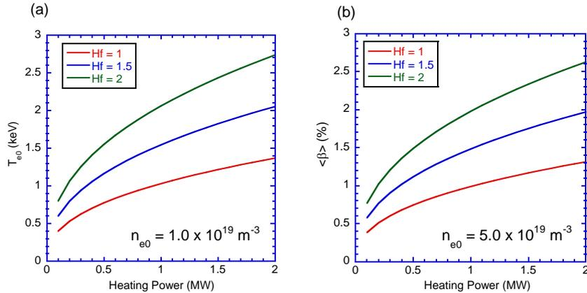
Figure 4. (a) Central temperature dependence on the heating power in CFQS estimated from ISS95 scaling low. (b) Volume averaged  $\beta$  dependence on heating power. For profiles,  $T = T_0 (1 - s)$ ,  $T_i = 0.75 T_e$ , and  $n = n_0 (1 - 0.8 s + 1.3 s^2 - 1.5 s^3)$  are assumed. Central electron density,  $n_0 = 1.0 \times 10^{19} \text{ m}^{-3}$  for (a) and  $5.0 \times 10^{19} \text{ m}^{-3}$  for (b).  $Hf$  is the improved factor from ISS95 scaling.
