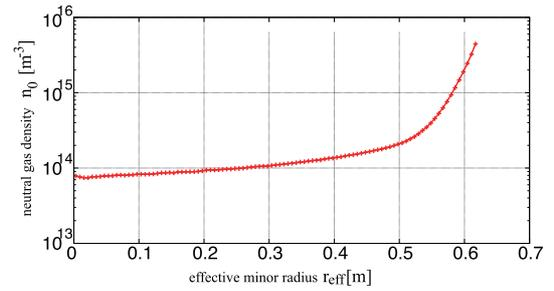
Fig. 4 The neutral gas density profile assumed in the simulation is shown. This profile is calculated by AURORA code [31] for the case in which the core electron density is approximately  $1.5 \times 10^{19} \text{ m}^{-3}$ . The plasma minor radius is approximately  $a = 0.61 \text{ m}$ .
