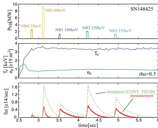
Fig. 2 The typical waveform of this series of experiments is shown. The injection powers and energies of NBs, the electron temperature and density on  $\rho = 0.5$ , and the neutron emission rate,  $S_n$ , are indicated. Solid and dashed curves in the bottom figure indicate the measured and simulated neutron emission rates. Simulation ignores the fast-ion loss.
