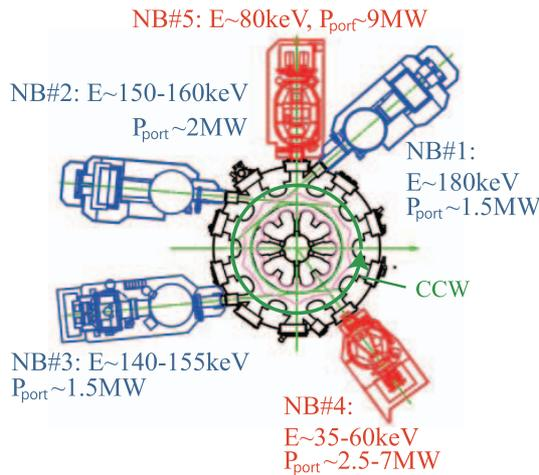
Fig. 1 The top view of the NBI system implemented in LHD is shown. NB#1-NB#3, which are the negative ion-based beams, are tangentially injected and, NB#4 and NB#5, which are positive ion-based beams, are perpendicularly injected. In this paper, the direction of the magnetic field line is counter-clockwise (CCW). Therefore, NB#1 and NB#3 are co-direction to the magnetic field line. Typical beam injection energies and powers are also displayed.
