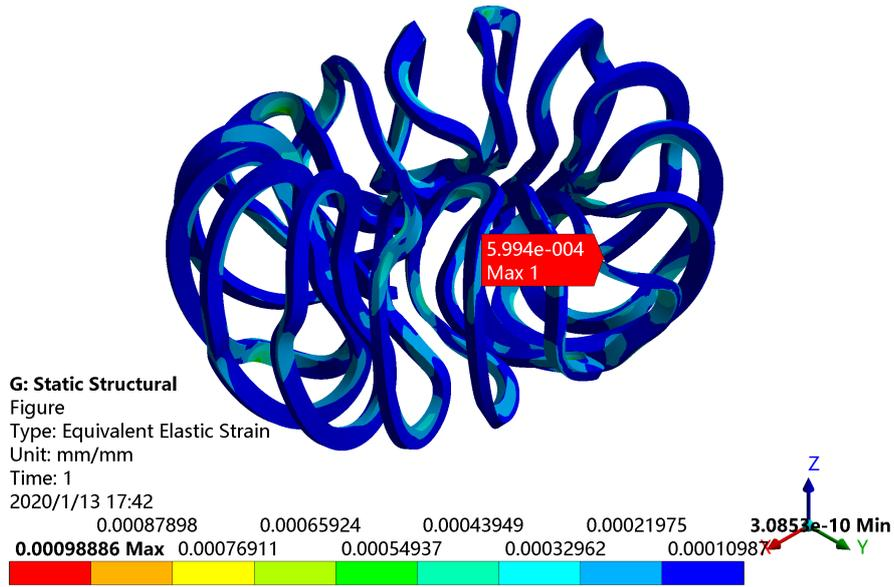
(c) Elastic strain distribution on winding packs (MC)
