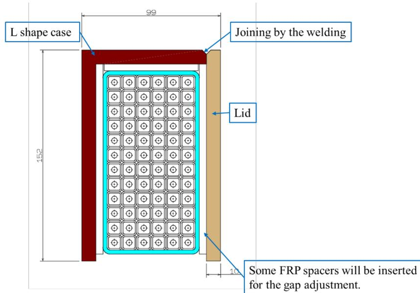
Figure 8. Design of the 'U' shape coil case.
