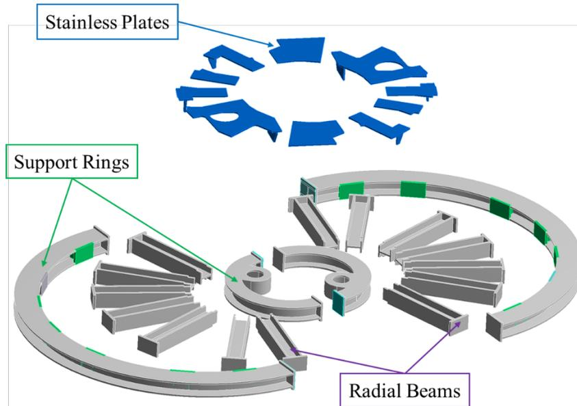
Figure 6. Detailed structure of top/bottom supports.
