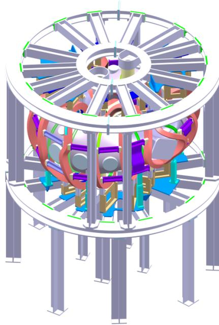
Figure 5. Overview of the supporting structure of CFQS.
