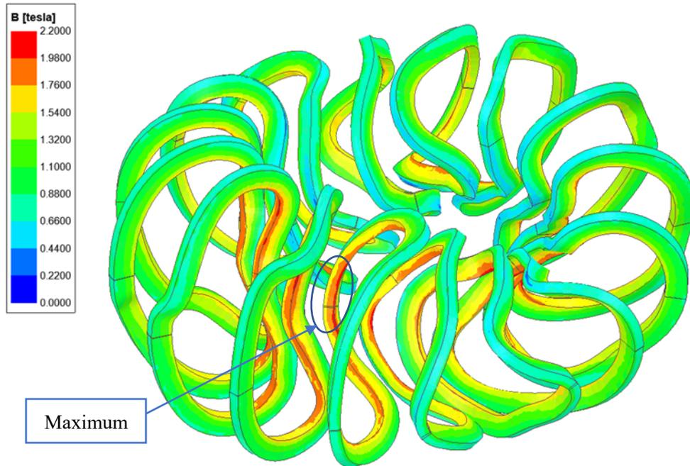
Figure 2. Magnetic field strength on modular coils.
