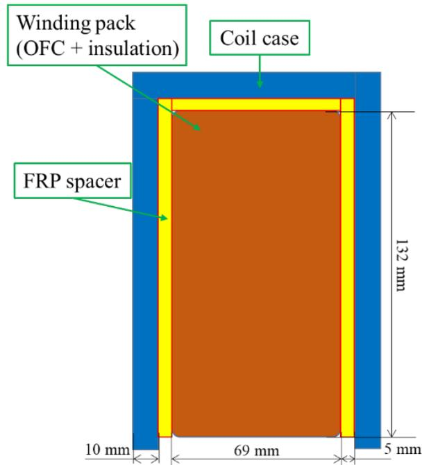
(c) Simplified cross-section of the winding pack
