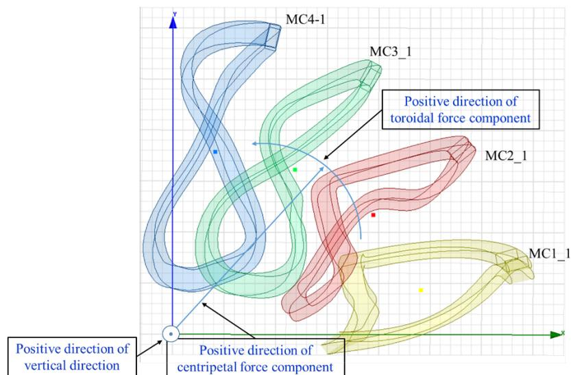
Figure 4. Definition of different EM force components.
