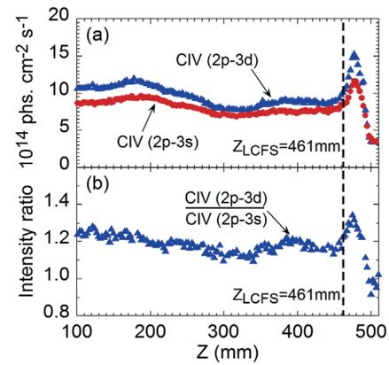
Fig. 6 Vertical profiles of (a) CIV 2p-3d ( $384 \text{ \AA}$ ) and 2p-3s ( $420 \text{ \AA}$ ) at  $\varphi = 0^\circ$  and (b) CIV line intensity ratio of 2p-3d/2p-3s. Position of LCFS is denoted with dashed line.
