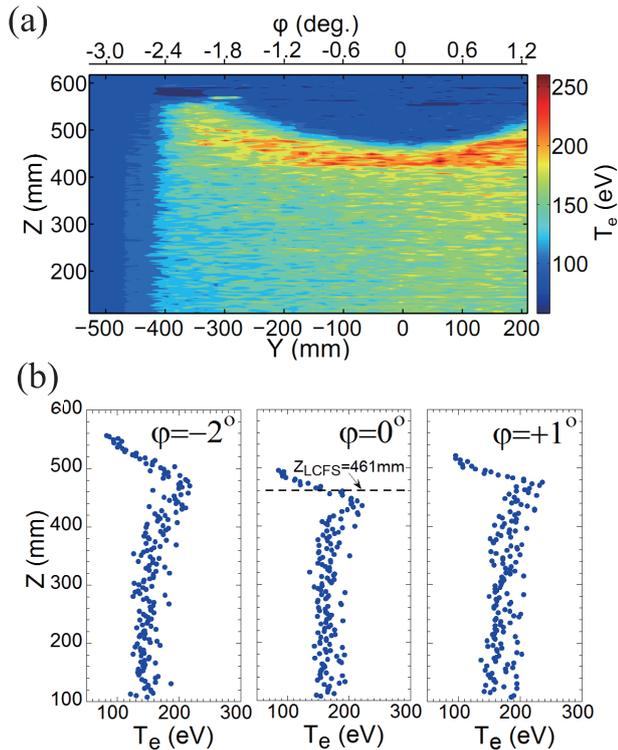
Fig. 5 (a) 2-dimensional distribution of edge  $T_e$  measured from NeVIII line intensity ratio and (b) vertical profiles of edge  $T_e$  at different toroidal positions of  $\varphi = -2^\circ, 0^\circ$  and  $+1^\circ$ . Position of LCFS is denoted with dashed line at  $\varphi = 0^\circ$ .
