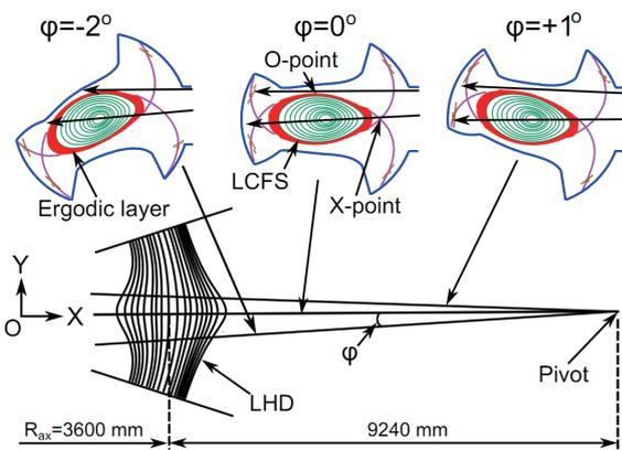
Fig. 1 Cross sections of LHD plasma at toroidal angles of  $\varphi = -2^\circ$ ,  $\varphi = 0^\circ$  and  $\varphi = +1^\circ$ . Two arrows indicate the observation range of space-resolved EUV spectrometer. The toroidal angle is defined as an angle from X-axis at the pivot of spectrometer. The vertical and horizontal spatial resolutions are  $\Delta Z = 10 \text{ mm}$  and  $\Delta Y = 80 \text{ mm}$ , respectively.
