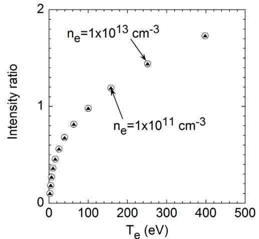
Fig. 4 Line intensity ratio of NeVIII 2s-3p ( $88 \text{ \AA}$ ) to 2p-3s ( $103 \text{ \AA}$ ) calculated by ADAS at electron densities of  $n_e = 1 \times 10^{11} \text{ cm}^{-3}$  (solid triangles) and  $n_e = 1 \times 10^{13} \text{ cm}^{-3}$  (open circles).
