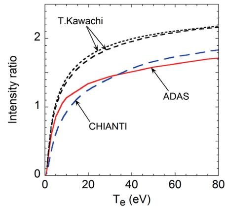
Fig. 7 Line intensity ratio of CIV 2p-3d ( $384 \text{ \AA}$ ) to 2p-3s ( $420 \text{ \AA}$ ) calculated by ADAS and CHIANTI at electron density  $n_e = 1 \times 10^{13} \text{ cm}^{-3}$  and T.Kawachi at  $n_e = 1 \times 10^{11} \text{ cm}^{-3}$  (long dash) and  $n_e = 1 \times 10^{13} \text{ cm}^{-3}$  (short dash).
