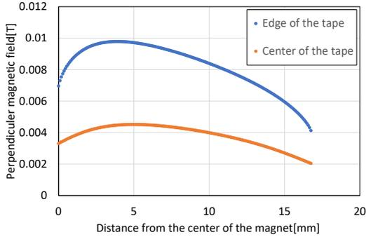
Fig. 5 Profiles of magnetic fields applied perpendicularly to the winding tape face.
