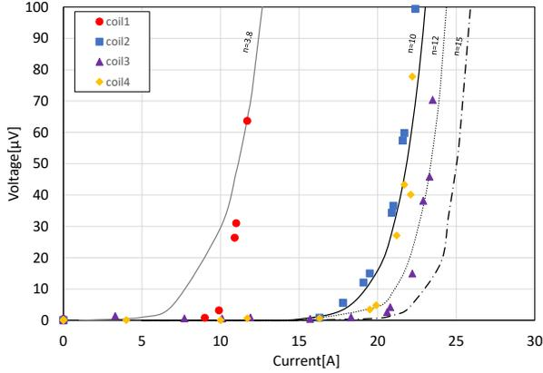
Fig. 4 I-V characteristics of the YBCO test coils and estimated I-V curve from n value model.
