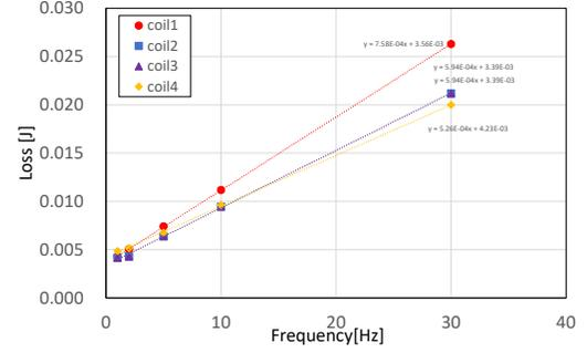
Fig. 6 Frequency dependencies of AC losses. (4 A[rms])
