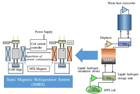
Fig. 1 An example of a liquid hydrogen recondensation system configuration using SMRS. superconducting coils.
