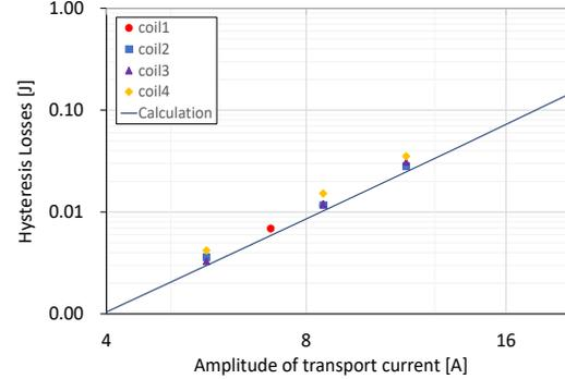
Fig. 7 Hysteresis loss for each coil and calculated loss from Norris's expression.
