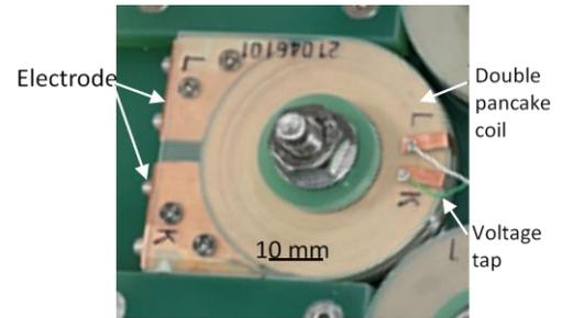
Fig. 2 Picture of YBCO test coil.
