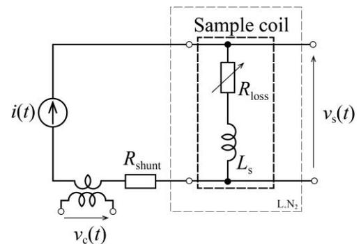
Fig. 3 Experimental circuit for AC loss measurement.  $R_{loss}$  is corresponding to ac losses in the sample coil. Inductive voltages in  $v_s(t)$  is canceled by using  $v_c(t)$ .
