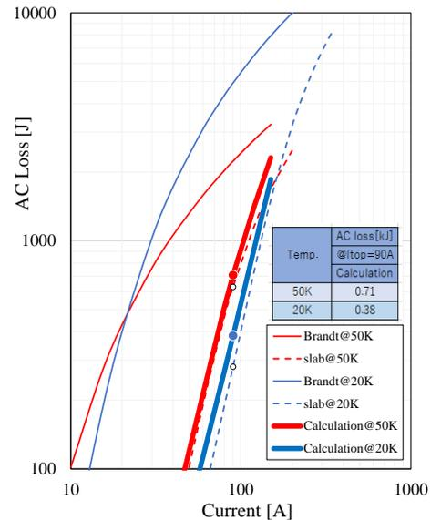
Fig. 9 AC loss calculation result for a HTS magnet of SMRS. Bold, solid and dashed lines represent Norris's expression, Brandt's expression and slab model, respectively. Red and blue represent 50K and 20K, respectively.
