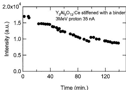
FIG. 4. Light output in the wavelength of 554 nm for  $Y_3Al_5O_{12}:Ce$  (sample 2) by 3 MeV proton beam irradiation at the temperature of 17 °C. The proton beam current of 35 nA is irradiated, and the flux corresponds to  $1.8 \times 10^{12}$  ions/( $cm^2$  s).
