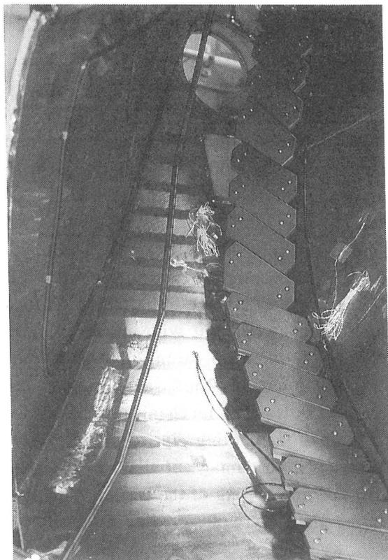
Fig. 1 Mock-up of an inside divertor unit
