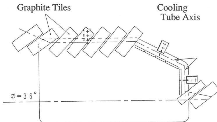
Fig. 2 An arrangement of the tiles at the opening of an upper port hole
