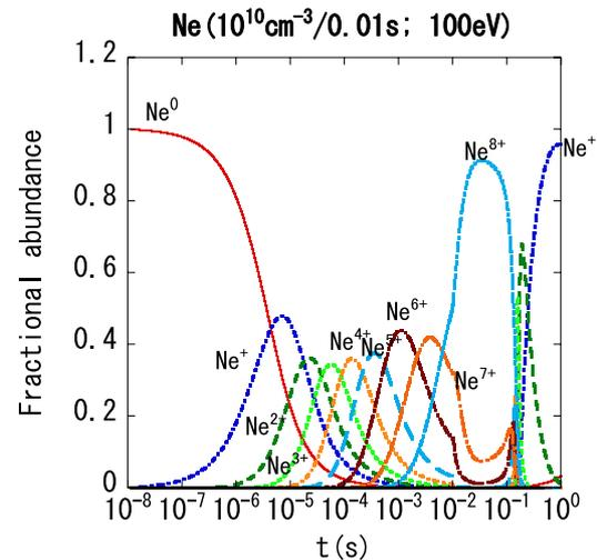
Fig. 6 Time evolution of fractional abundance for the case with  $(R_{\text{puff}} = 10^{12} \text{ cm}^{-3} \text{ s}^{-1})$  and  $T_e(0) = 100 \text{ eV}$  (case g).
