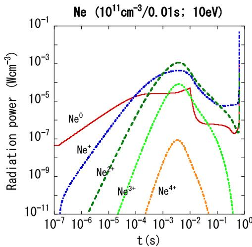
Fig. 4 Time evolution of radiation power due to each ion for the same case as in Fig. 1 (case a).
