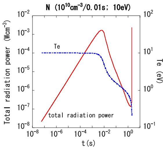
Fig. 8 Time evolution of total radiation power and electron temperature for nitrogen case with  $R_{\text{puff}} = 10^{12} \text{ cm}^{-3}$  and  $T_e(0) = 10 \text{ eV}$ .
