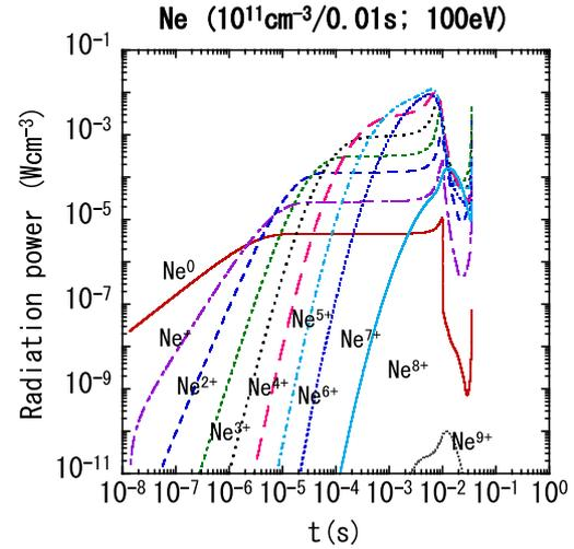
Fig. 5 Time evolution of radiation power due to each ion for the case c with  $R_{\text{puff}} = 10^{13} \text{ cm}^{-3} \text{ s}^{-1}$  and  $T_e(0) = 100 \text{ eV}$  (case c).
