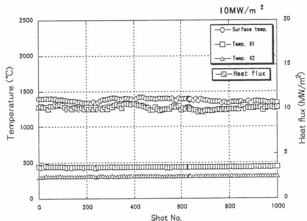
Fig.3 Relationship between the temperatures of a mock-up and the shot number of a cyclic heat load of 10 MW/m<sup>2</sup>.
