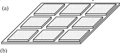
Figure 1. (a) Drawing of double layer foil with SS base (grey) and gold absorber (gold). (b) Cross-section of double layer foil showing perforation in SS under gold absorber.
