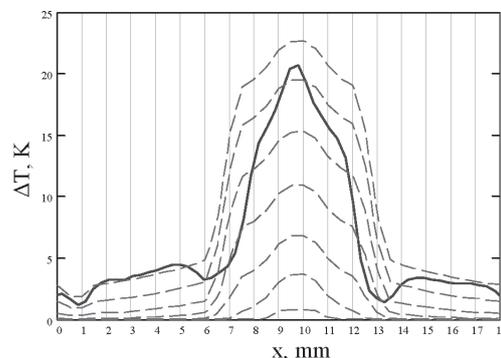
Figure 3. Temperature profile evolution of DLF from FEM (red dashed) at 2.5, 25, 100, 250, 500, 1000, 2500 ms after exposure to laser compared with measured DLF temperature profile at 2500 ms (blue solid).
