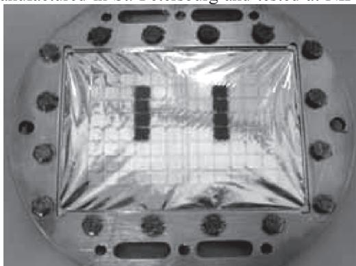
Figure 2. Prototype of a DLF with 2.1 micron and 0.85 micron gold absorbing layers and a 2.5 micron SS base. Some pixels are blackened with graphite to increase the IR emissivity.
