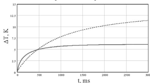
Figure 4. Measured temperature evolution of DLF (dashed) after exposure to laser compared with that of single layer gold foil (solid).
