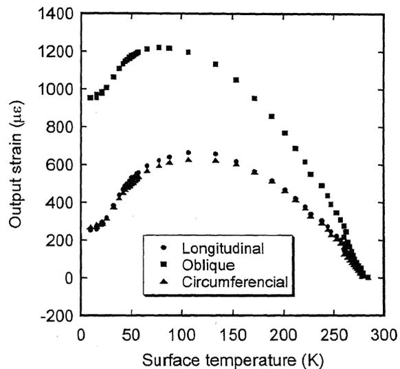
Fig. 7. Apparent strain against temperature obtained from strain gauges on the reinforced Bi-2212 specimen.
