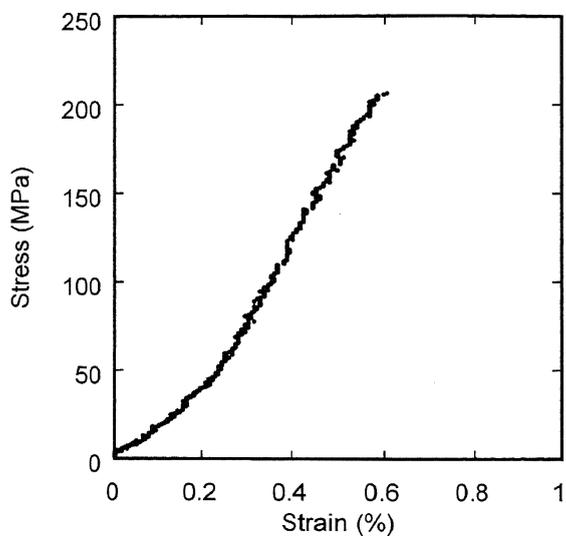
Fig. 3. Stress-strain curve of Bi-free substrate at room temperature.
