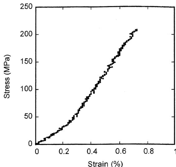
Fig. 2. Stress-strain curve of Bi-2212 tubular bulk at room temperature.
