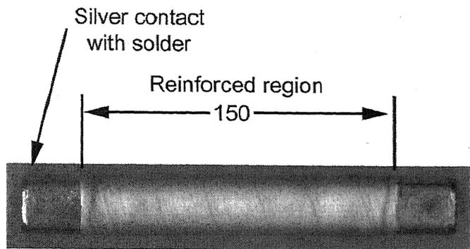
Fig. 6. Bi-2212 tubular bulk with glass-epoxy reinforcement.
