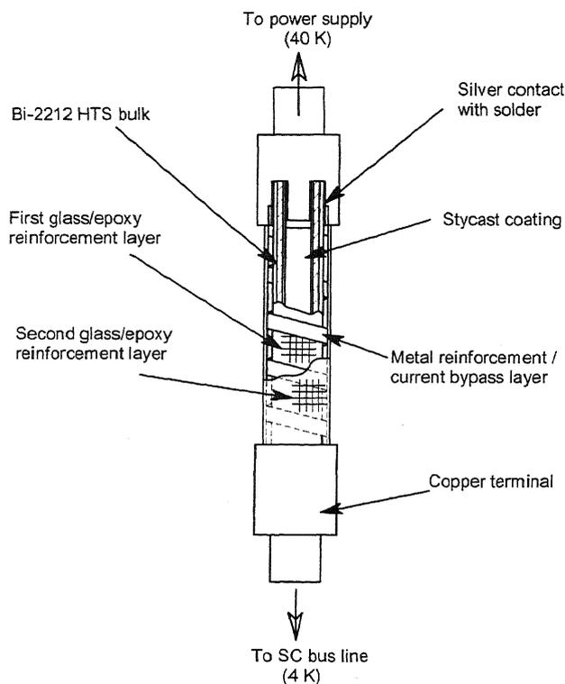
Fig. 8. Example design of current lead using Bi-2212 tubular HTS.
