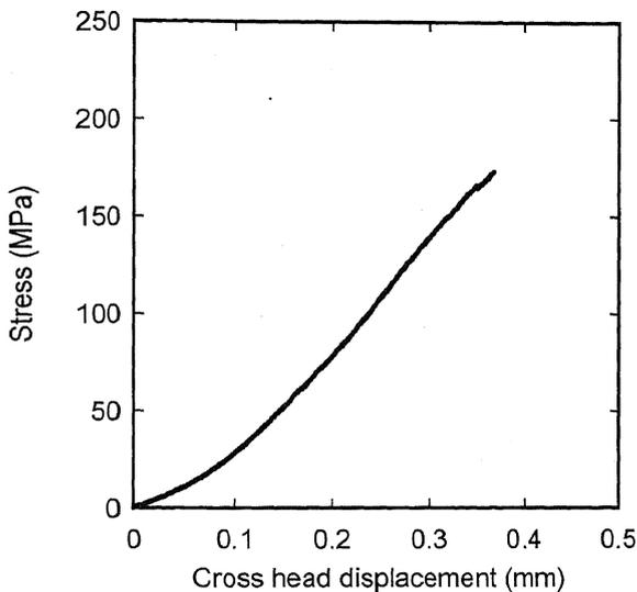
Fig. 5. Stress against cross head displacement of Bi-free substrate at 77 K.
