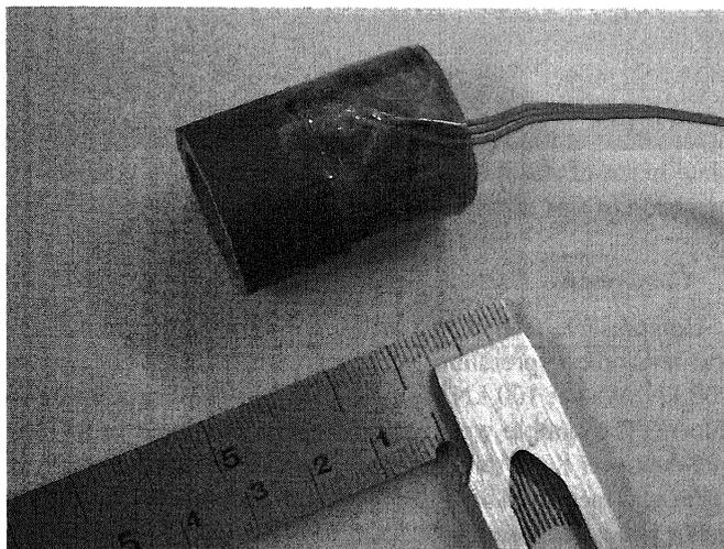
Fig. 1. A specimen for thermal contraction and compressive test.
