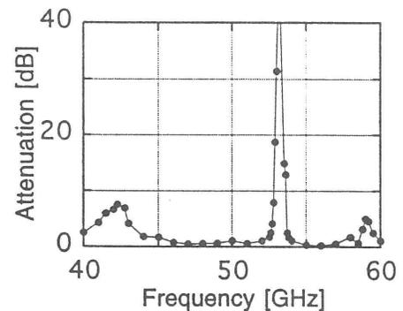
Fig.2. Attenuation data of the band rejection filter
