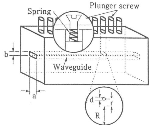
Fig.1. Outward form of the band rejection filter
