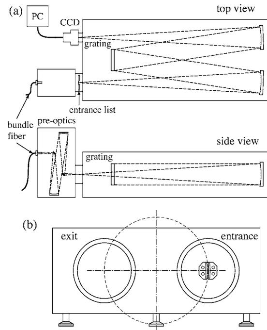
FIG. 2. Schematic geometry of (a) the spectrometer and preoptics and (b) the circular curved entrance slit. The preoptics are topologically similar to the spectrometer: the focal length of the spherical mirrors is 300 mm, while it is 1.33 m for the spectrometer.
