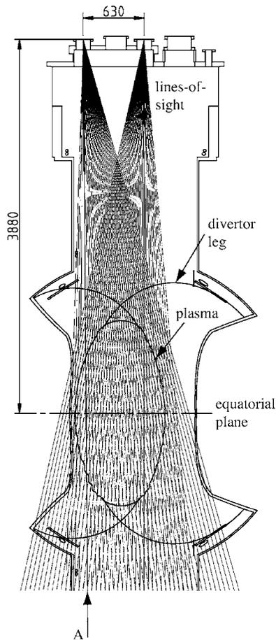
FIG. 1. Cross section of the vacuum vessel and the elliptical plasma for the observation. The major radius of the vacuum vessel center is 3.9 m. The plasma is observed with two arrays of optical fibers. Each array consists of 40 channels. The spectrum shown in Fig. 4 is obtained with the line-of-sight "A" in this figure.
