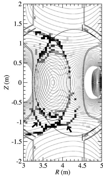
FIG. 5. Obtained Emission locations with all the lines of sight as a result of tomographic analysis. The darkness corresponds to the line intensity. The radiation regions indicated with the arrows seem to be ghosts which have wrongly survived the tomographic analysis.
