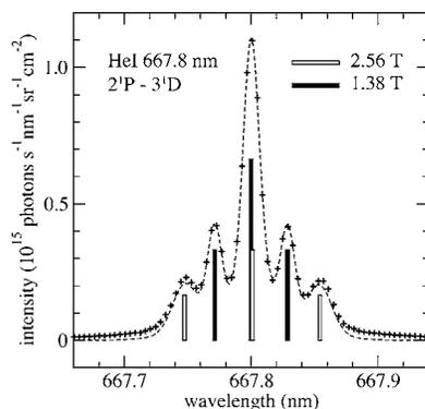
FIG. 4. Measured spectrum for the He I  $\lambda 667.8\ \text{nm}$  line with the line-of-sight “A” indicated in Fig. 1. The profile is well fitted with two Zeeman components and field strengths of 2.56 and 1.38 T are derived.
