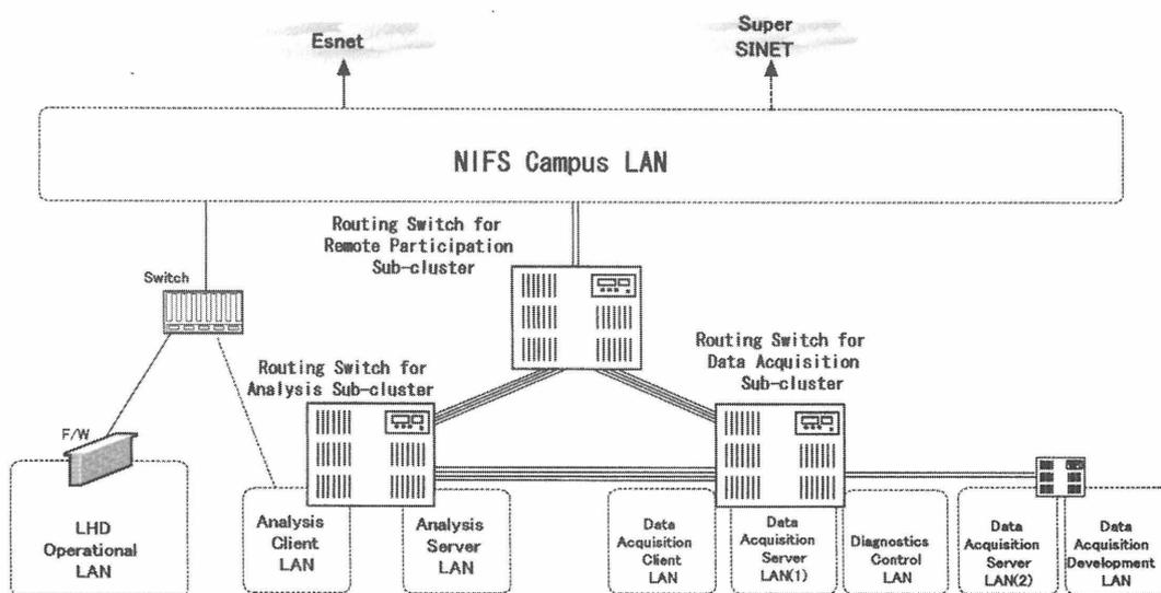
Fig. 1 Block diagram of new LHD-LAN
