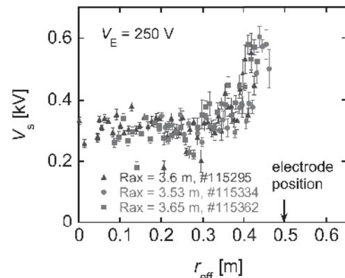
Fig. 3 Space potential profiles measure by HIBP
