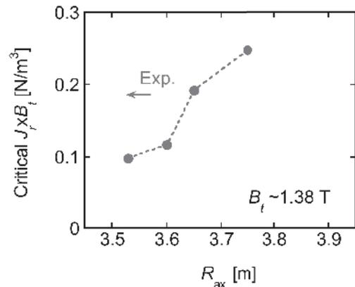
Fig. 2 Dependence of the external driving force  $\mathbf{J} \times \mathbf{B}$  required for the improved mode transition (critical driving force) on configuration
