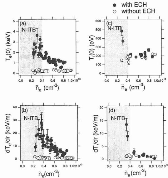
Fig. 1: Central electron (a) and ion (c) temperature and electron temperature gradient (b) and ion temperature gradient (d) as a function of line averaged density. The close circles denote the plasma with ECH. The open circles denote the plasma without ECH.
