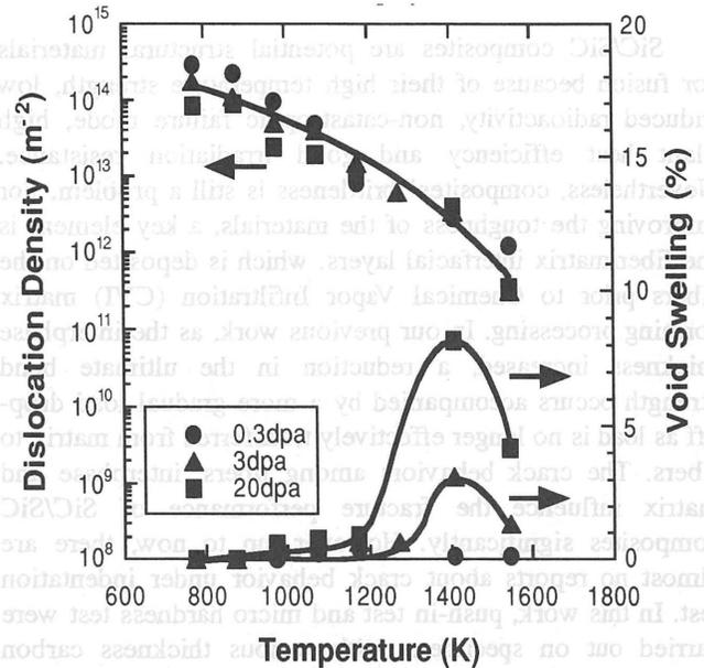
Fig.1. Temperature dependence of dislocation density and swelling.
