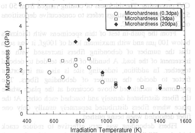
Fig.2. Temperature dependence of the hardness measured by the micro-indentation technique.
