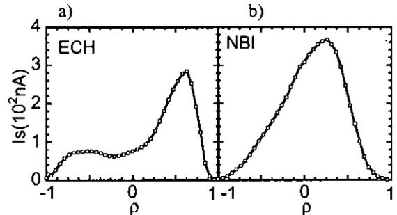
Fig.1 a) Profiles of secondary beam current from ECH plasma and b) from NBI plasma
