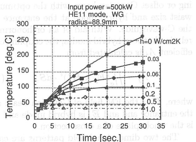
Figure 1 Calculated results of time evolution of the peak temperature during 84GHz, 500kW, HE<sub>11</sub> mode injection to the Brewster window with forced air cooling. Disk material is a low-loss silicon nitride composite.
