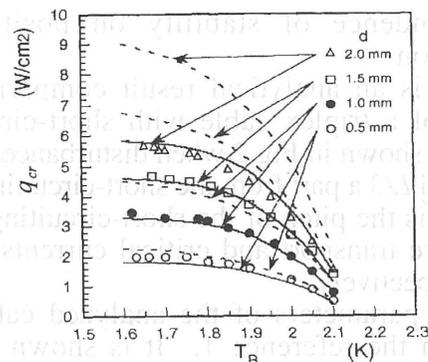
Fig.2 Critical heat flux versus bulk liquid temperature with channel gap as a parameter.
