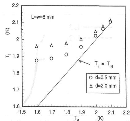
Fig.3 Channel entrance liquid temperature at CHF versus bulk liquid temperature.
