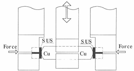
Figure 1: Experimental arrangement.
