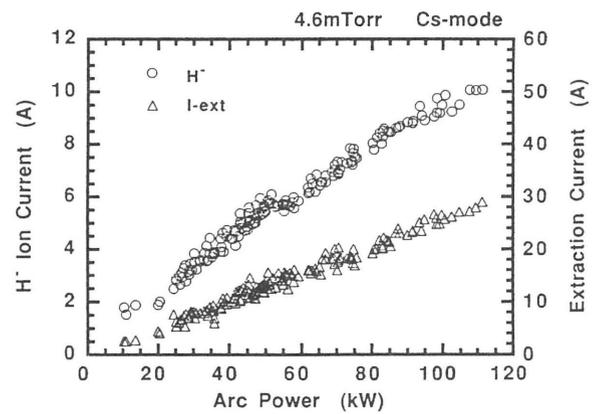
Fig. 2. Negative ion and the extraction currents as a function of the arc power. The gas pressure is 4.6 mTorr.
