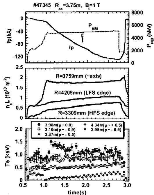
Fig.1 Time evolution of electron density and electron temperature at various radial location with large reversed current  $I_p$  up to 130 kA, where  $B_t=1T$ , magnetic axis position  $R_{ax}=3.75m$ , and absorbed NBI power is 5MW. Neon puff is applied at  $t=0.9s$ .
