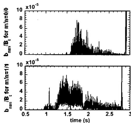
Fig.2 Time evolutions of magnetic fluctuations with  $m/n=0/0$  and  $1/1$  mode structure in the shot shown in Fig.1.
