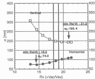
Fig. 3. Horizontal and vertical beam width as functions of the voltage ratio  $R_v$ . The plots with closed circles and open squares are changes of horizontal and vertical changes of beam widths, respectively.
