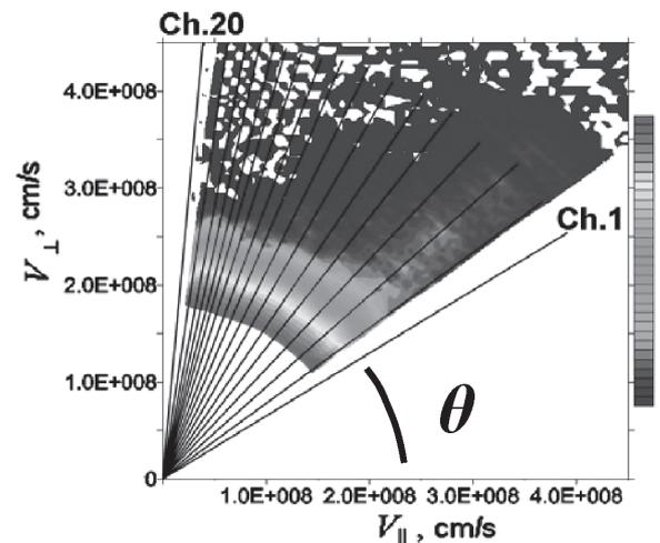
Fig.2 Energy spectrum measured along 20 sightlines. ( $\theta$  is the angle between the sightline and magnetic axis)
