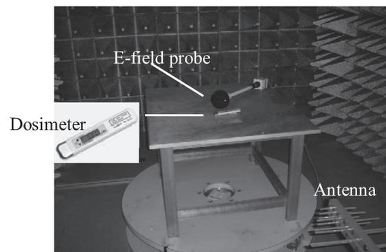
Fig. 1 View of measurement for susceptibility of personal dosimeter
