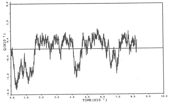
Fig.2. The temporal charging process of the grains when the secondary electron emission effect is taken into account.
