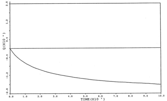
Fig.1. The temporal charging process of the grains when the secondary electron emission effect is neglected.
