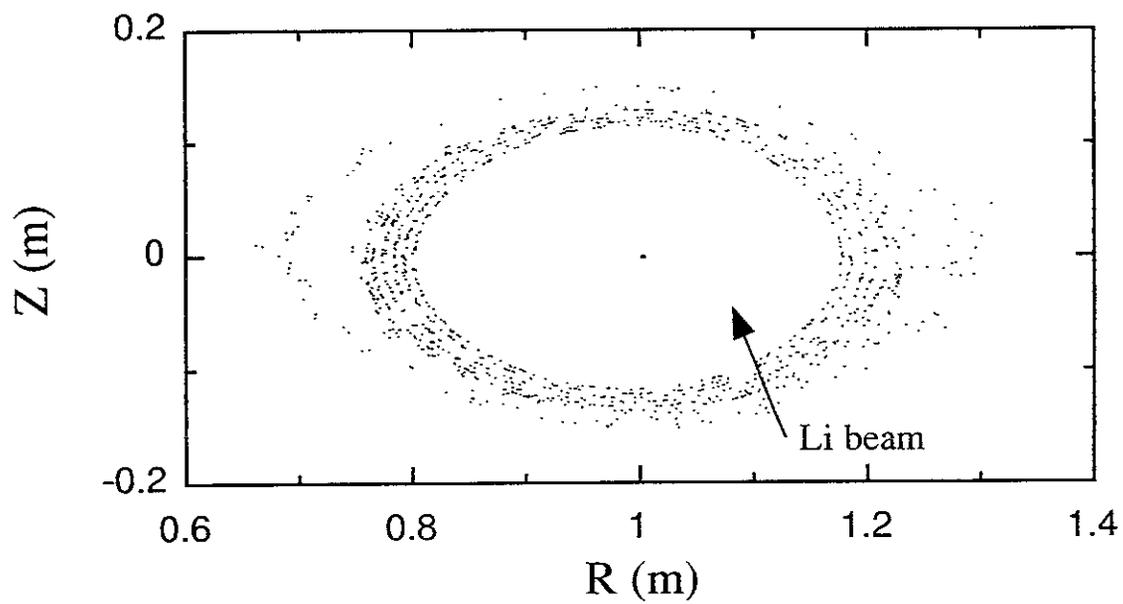
Fig. 4 Magnetic configuration with the 1/1 island in the poloidal plane at Li beam probe.
