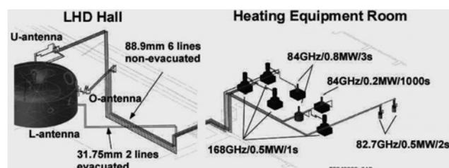
Fig. 1 ECH system in LHD, which consists of 82.7 GHz, 84 GHz, 168 GHz gyrotrons, transmission lines and antennas.
