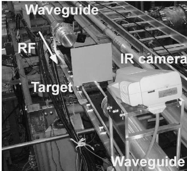
Fig. 7 Configuration of IR pattern measurement system mounted in the transmission line. Waveguide axis is adjusted to coincide with the target center by visible lasers.
