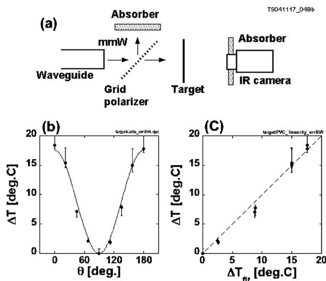
Fig. 6 (a) Schematic diagram of a test setup for the millimeter-wave absorption in the target to assure the linearity of the temperature rise on irradiated power. Measured temperature increase  $\Delta T$  is plotted as a function of the polarizer angle  $\theta$  in (b). In (c) the measured  $\Delta T$  is plotted versus the fitted temperature increase  $\Delta T_{\text{fit}}$  that is in proportion to the irradiated power on the target.
