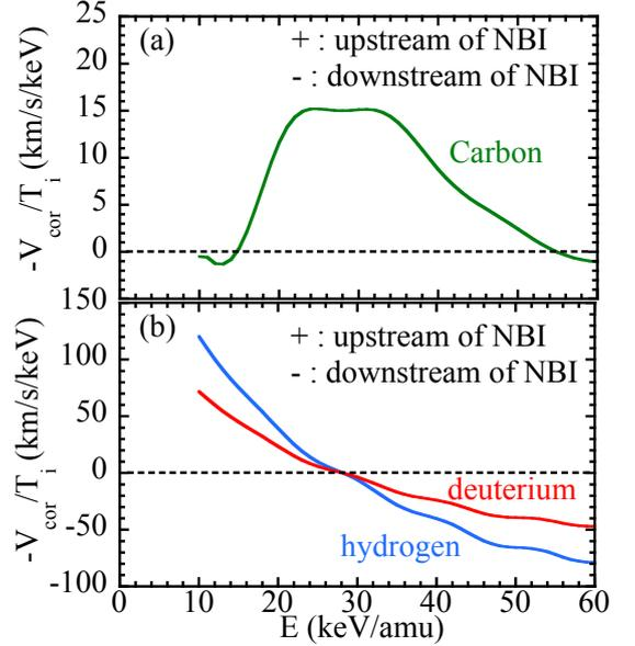
FIG. 4: Correction coefficient of toroidal velocity due to cross section effect on (a) carbon and (b) hydrogen and deuterium as a function of beam energy per atomic unit. Here the fraction of  $n = 2$  excited state is 0.2%.
