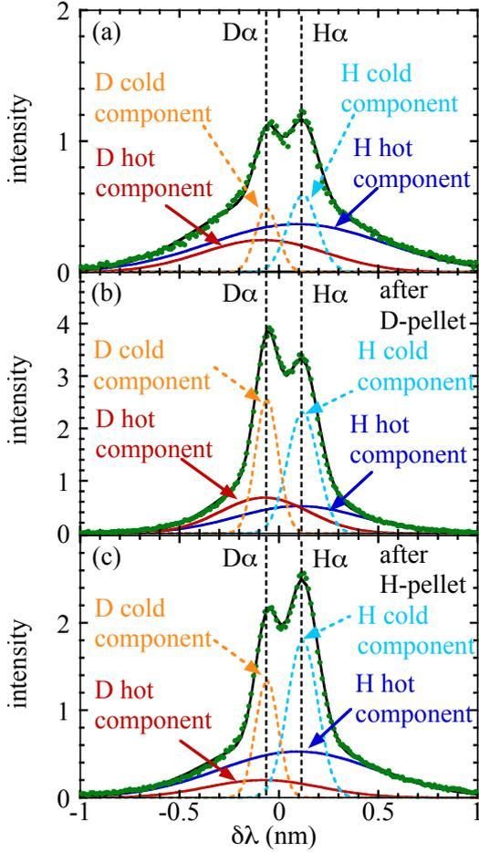
FIG. 3:  $H\alpha$  and  $D\alpha$  spectrum (a) before pellet injection, (b) after deuterium pellet injection, and (c) after hydrogen pellet injection.
