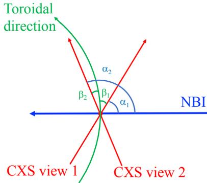
FIG. 1: Experimental set up: geometry of neutral beam, line of sight of bulk charge exchange spectroscopy.
