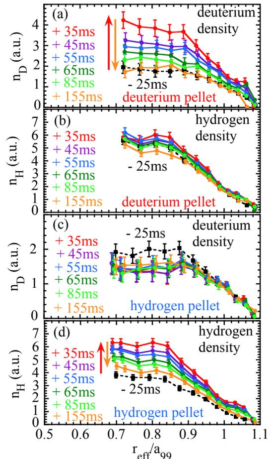
FIG. 9: Radial profile of (a)(c) deuterium and (b)(d) hydrogen density in the plasma with (a)(b) deuterium and (c)(d) hydrogen pellet injection.
