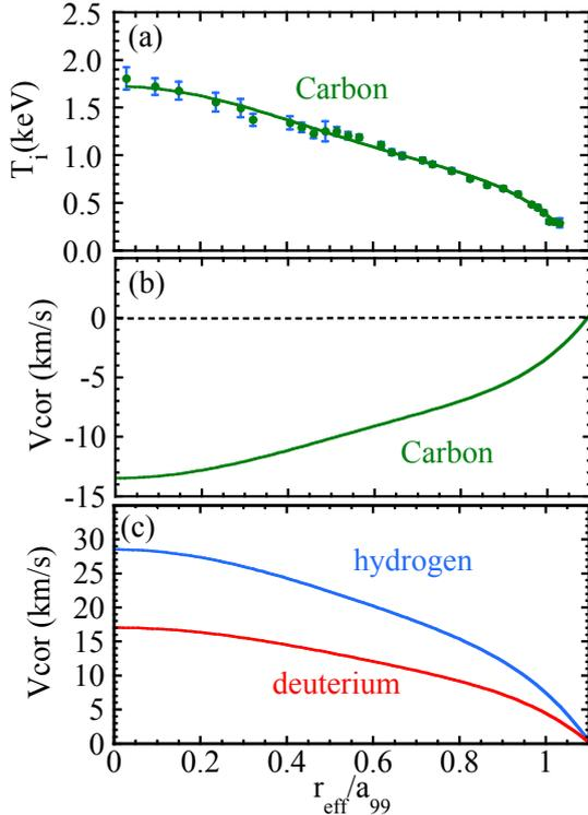
FIG. 5: Radial profile of (a) ion temperature of carbon and atomic correction of toroidal rotation for (b) carbon ion, (c) hydrogen, and deuterium ions. Here positive velocity is red shift and negative velocity is blue shift. Here the beam species is hydrogen and beam energy is 43 keV/amu.
