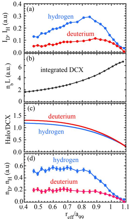
FIG. 8: Radial profile of (a) intensity of deuterium and hydrogen hot component, (b) line integrated beam density, (c) the ratio of Halo contribution to direct change exchange (DCX) contribution, and (d) density of deuterium and hydrogen.
