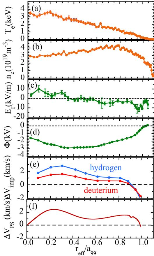
FIG. 6: Radial profile of (a) electron temperature, (b) electron density, (c) radial electric field, (d) space potential, (e) velocity differences between hydrogen or deuterium bulk ions and carbon impurity ion calculated by DKES code, and (f) velocity difference of Pfirsch-Schlüter flow between bulk ions and carbon impurity ion calculated. Here positive velocity is in co-direction and negative velocity is in counter-direction.
