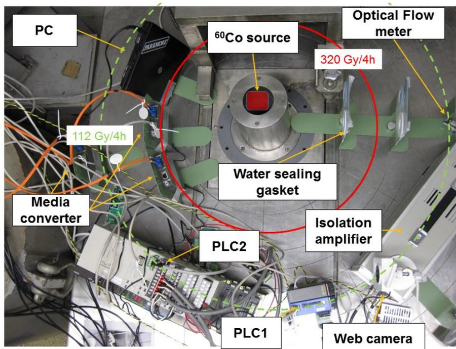
Fig.1 Experimental setups for gamma-ray irradiation
