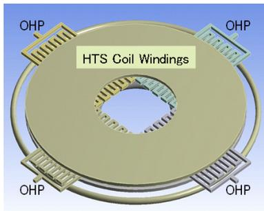
Fig. 4 OHP built in element HTS coil
