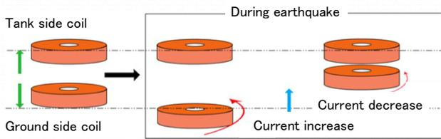
Fig. 2 Base-isolated control using an HTS coil pair
