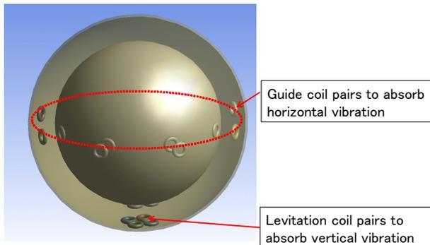
Fig. 3 Magnetic levitation image of a 40-m-diameter LH<sub>2</sub> storage tank
