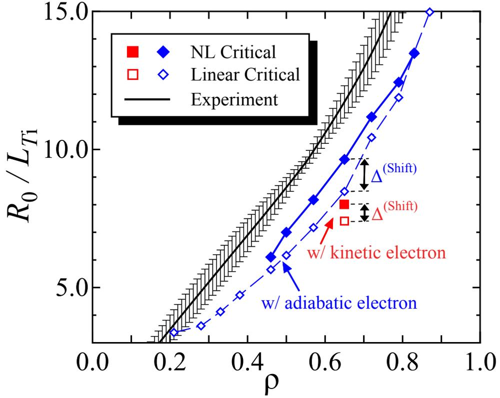
FIG. 3. Radial profile of the critical ion temperature gradient obtained from the simulation with kinetic electrons (red) and adiabatic electrons (blue). Filled symbols represent the nonlinear results and open symbols are linear results linear results, and  $\Delta^{(\text{shift})}$  correspond to Eq.(4). Black curve and errorbars show the radial gradients of the ion temperature from the experiment which will be discussed in Sec.IV.
