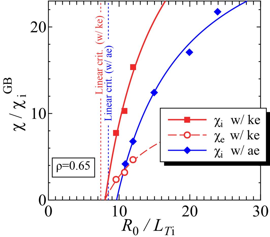
FIG. 2. The ion temperature gradient dependencies of the heat transport coefficients for ion (red squares) and electron (red circles) from electromagnetic gyrokinetic simulations with kinetic electrons at  $\rho = 0.65$  in the LHD high- $T_i$  plasma. Here,  $\chi_i^{GB} = \rho_{ti}^2 v_{ti} / R_0$ . Blue diamonds represent the ion heat transport coefficients from electrostatic simulations with adiabatic electrons. Dotted lines are the critical temperature gradients from linear analyses.
