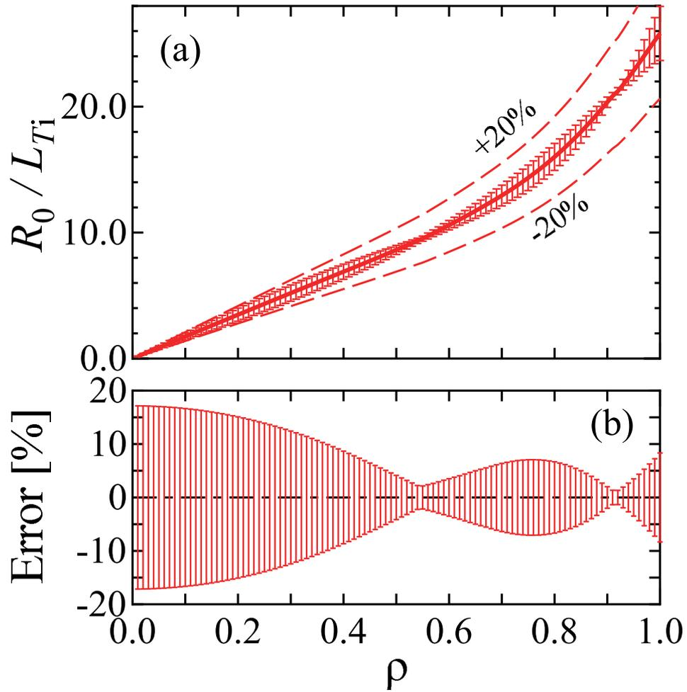
FIG. 7. The radial profile of (a) the radial gradients of the ion temperature with the ranges from the AIC theory, and (b) the relative error level of the ranges. In the top figure,  $\pm 20\%$  of the medians of the temperature gradients are shown by the dashed curves.
