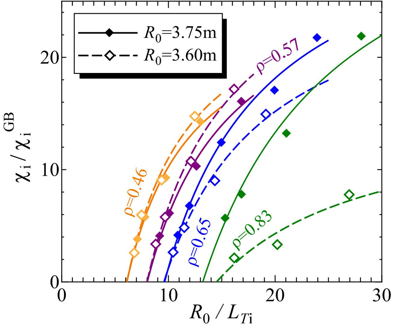
FIG. 4. The ion temperature gradient dependences of the ion heat transport coefficients at each radial position,  $\rho = 0.46, 0.57, 0.65$  and  $0.83$  in the standard LHD case with  $R_0 = 3.75\text{m}$  (solid curves) and the inward shifted LHD case  $R_0 = 3.6\text{m}$  (dashed curves).
