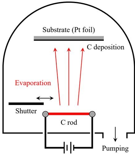
FIG. 2. (Color online). Schematic of evaporation coating.
