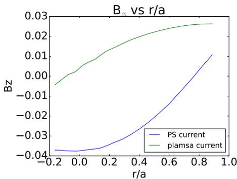
**FIG. 2.** The profile of  $B_z$  along the sightline of the diagnostic is plotted. The plasma current contribution to  $B_z$  goes to zero in the core but the slope with respect to flux is nonzero. The PS current current is nonzero in the core but the slope is approximately equal to zero in the core. Therefore using the derivative of  $B_z$  with respect to flux can minimize the effect of the uncertainty in PS current on the analysis.
