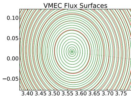
**FIG. 7.** The change in the flux surfaces with the new mapping are plotted. The new flux surfaces in green have a much finer resolution in the core than the old mapping, in red. The plots show mode amplitudes as a function of flux for the two mappings.
