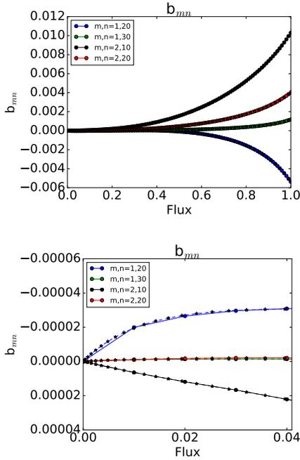
**FIG. 6.** The mode amplitudes of the VMEC outputs were interpolated in mode spaces using a Chebshev fit starting from equidistant points in flux space to equidistant in  $r/a$  space in order to increase the core resolution of the VMEC database. The stars are the interpolated fits while the circles are the original data.
