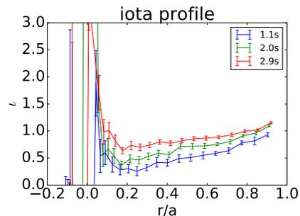
**FIG. 1.** The old fitting routine often gave unphysical values of the iota profile in the core region due to uncertainties in the PS contribution to the MSE measurement. Beyond  $r/a$  values of .3, where the relative contribution of the PS current is smaller, the fitting routine works well and the change in iota with a change in current is recoverable.
