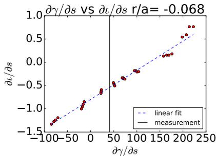
**FIG. 5.** The VMEC database is used to find the change in polarization angle and iota with respect to flux. This is calculated for a scan of currents and current profiles and a linear fitting is done to find the experimental change in  $d\iota/ds$  from a given MSE measurement of  $d\gamma/ds$ . The vertical line is the experimentally measured  $d\gamma/ds$  value. The very hollow profiles can have a nonlinear dependency and are therefore ignored in the fitting.
