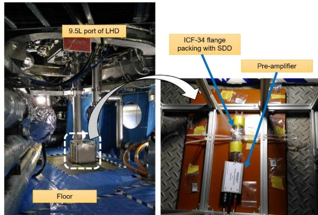
**Figure 2.** Picture of SDD set underneath 9.5L port of LHD in the torus hall.
