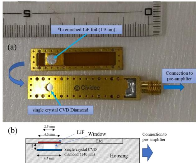
**Figure 1.** (a) the picture of SDD with the lid pasted with 1.9 μm LiF, (b) the schematic view of the cross-section of SDD
