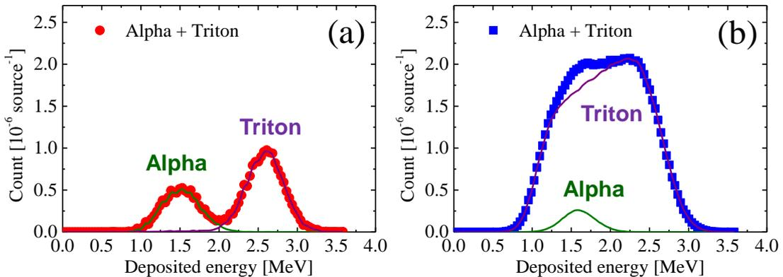
**Figure 6.** The PHS of SDD with (a) 1.9  $\mu\text{m}$  LiF and (b) 350  $\mu\text{m}$  LiF estimated by PHITS.
