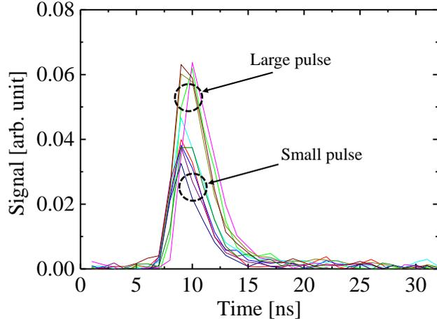
**Figure 3.** Typical signals from SDD with 1.9  $\mu\text{m}$ -thick LiF
