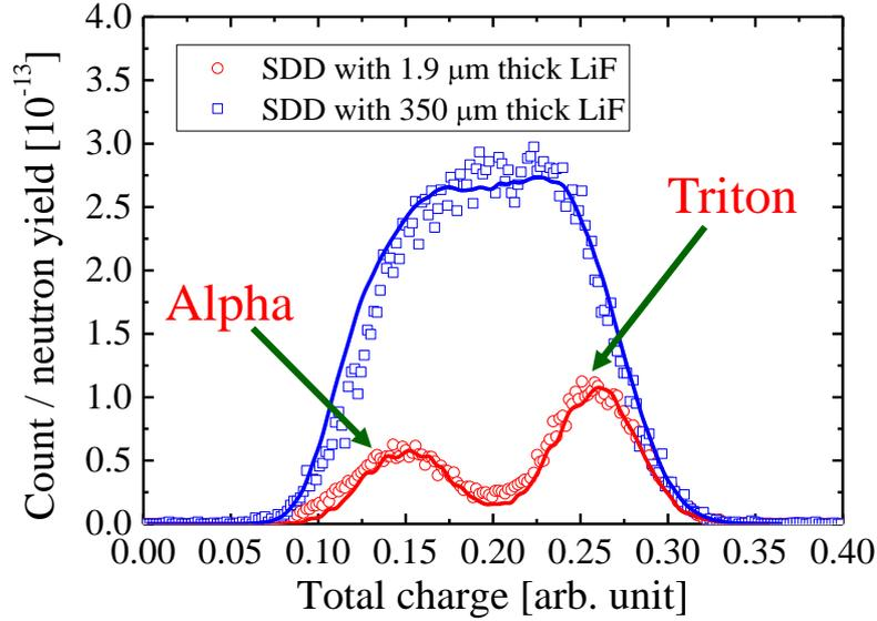
**Figure 5.** PHS for SDD with LiF with different thicknesses. The solid lines in each case are the PHS spectra of energetic particles (alpha + triton) evaluated by PHITS as same as Fig. 6.
