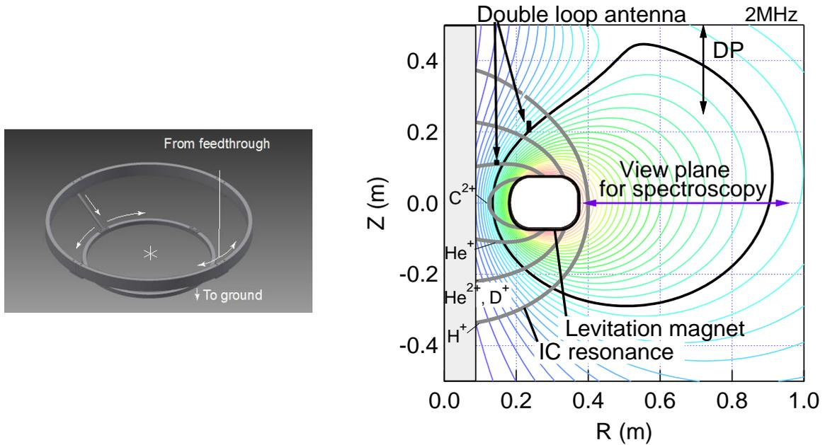
Figure 2. Double-loop antenna and the current direction (left figure). Poloidal cross-section of RT-1 with ion cyclotron resonance layers for main and impurity ions in the case of RF frequency of 2 MHz, and Poloidal field lines. DP is the probe position for edge electron temperature measurement. The position of the double loop antenna is indicated.
