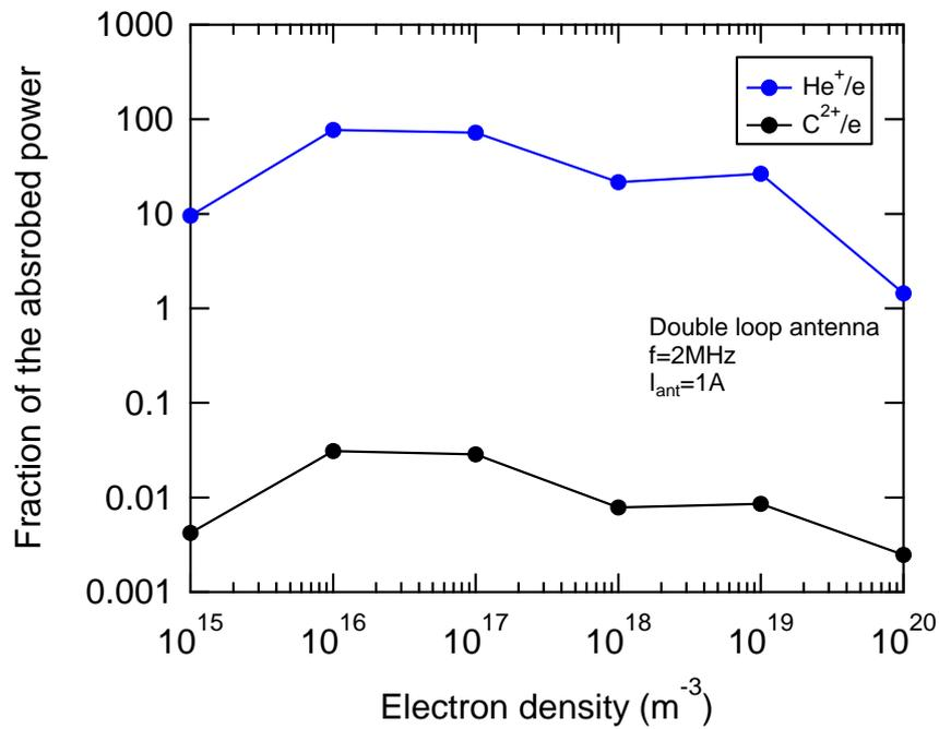
Figure 3. A fraction of the absorbed powers for He<sup>+</sup> and C<sup>2+</sup> normalized by that for electron calculated with electrons, helium ions (He<sup>+</sup>: 99%), and carbon impurities (C<sup>2+</sup>: 1%) as a function of the electron density in the case of the double-loop antenna. The antenna current of 1 A with the frequency of 2 MHz is applied to the double-loop antenna.
