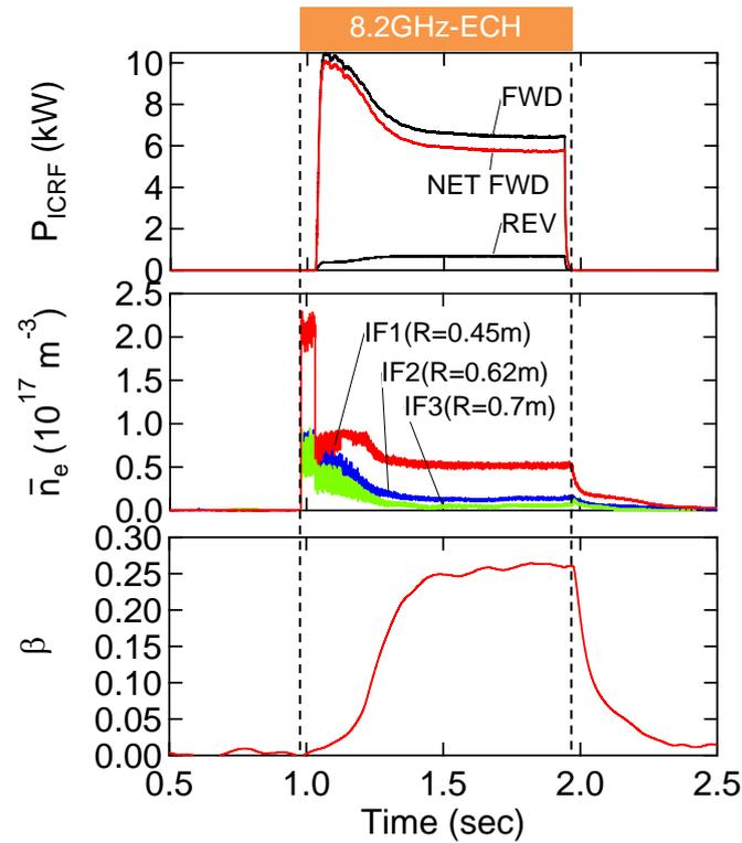
Figure 4. Time evolutions for ICRF forward and reflected powers, line averaged densities  $\bar{n}_e$ , and local electron  $\beta$  for ICRF heating in high  $\beta$  helium plasma. The target plasma is sustained by 8.2 GHz EC heating. The ICRF power is applied to the double-loop antenna immediately after the start-up of the ECH.
