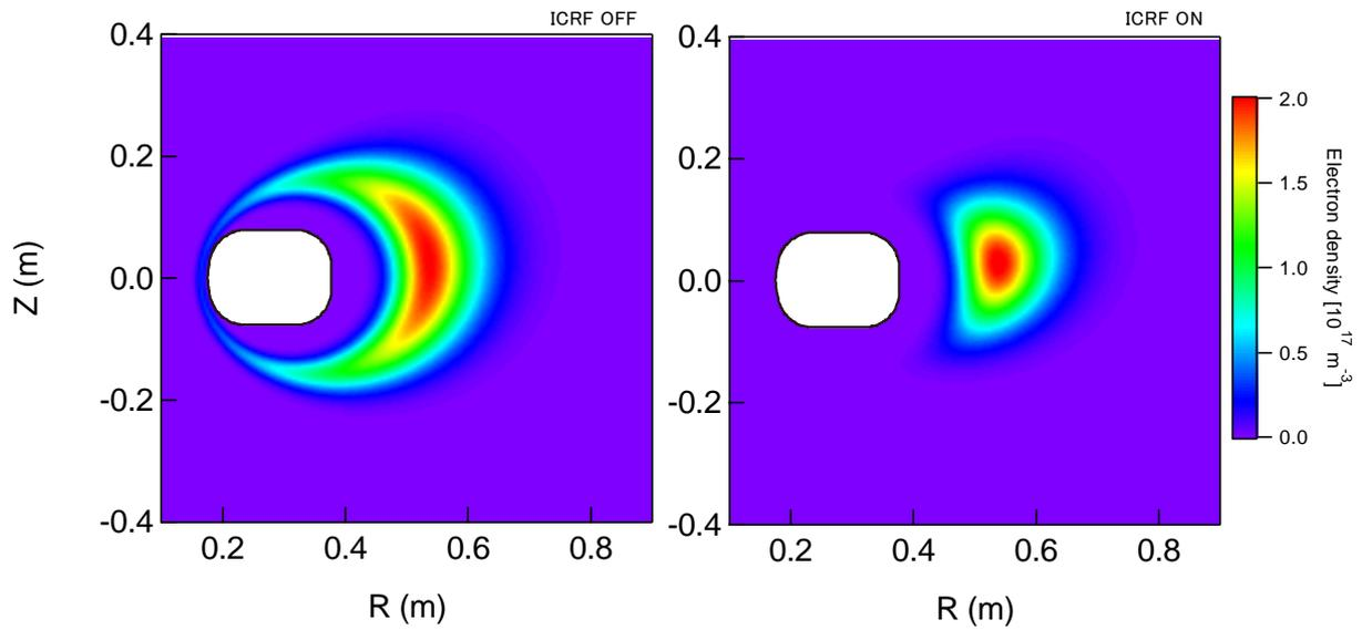
Figure 7. Change in the electron density profiles during the ICRF heating in the RT-1. ICRF heating is turned off (left) and on (right). Density profiles are reconstructed using the data measured by interferometers and DP.
