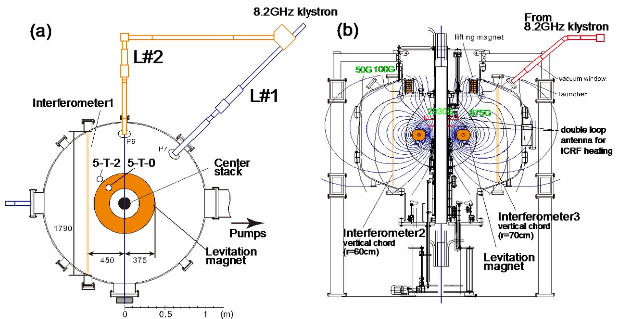
Figure 1. (a) Top and (b) cross sectional views of RT-1. Transmission lines L#1 and L#2 for 8.2-GHz EC heating and three interferometer cords are shown. (c) Double loop antenna used for ICRF heating.
