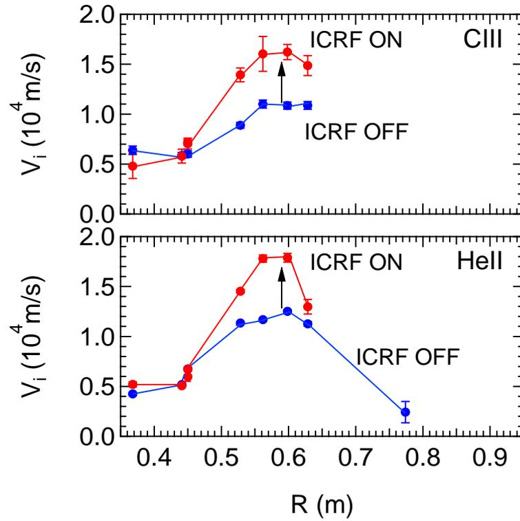
Figure 6. Radial profile of ion flow velocity for C III and He II on the equatorial plane of RT-1 in helium plasmas for the ICRF heating ON (in red) and OFF (in blue). The measured data were accumulated over the time period from 1.5 to 2.0 s.
