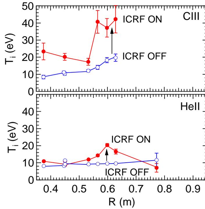
Figure 5. Radial profile of ion temperatures for C III and He II on the equatorial plane of RT-1 (see in figure 2) in helium plasmas for the ICRF heating ON (in red) and OFF (in blue). The measured data were accumulated over the time period from 1.5 to 2.0 s.
