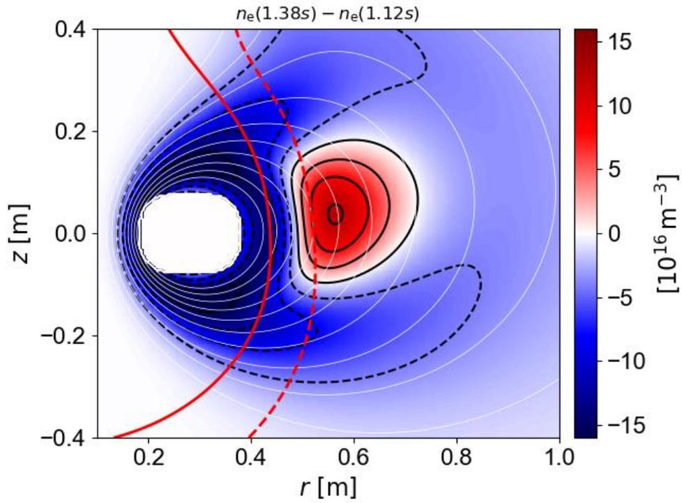
FIG. 4. Difference of the electron density. The reconstructed density profile at  $t = 1.38$  s is subtracted from that at  $t = 1.12$  s. The increase in the density is observed at  $r = 0.55$  m. The locations for the fundamental and the second harmonic resonances are indicated by the solid and the broken curves in red.
