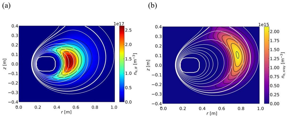
Fig. 2. Measured profiles of (a) the electron density and (b) the high-energy electrons. The spontaneous belt structure of high energy electrons is observed in outer radial location.
