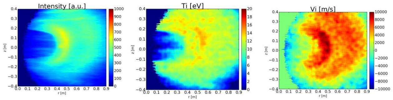
FIG. 6. Line-integrated emission intensity, temperature, and flow velocity of He<sup>+</sup> in the case of ICRF off (upper row) and on (lower row). The ICRF heating increases the He<sup>+</sup> intensity and the ion temperature.
