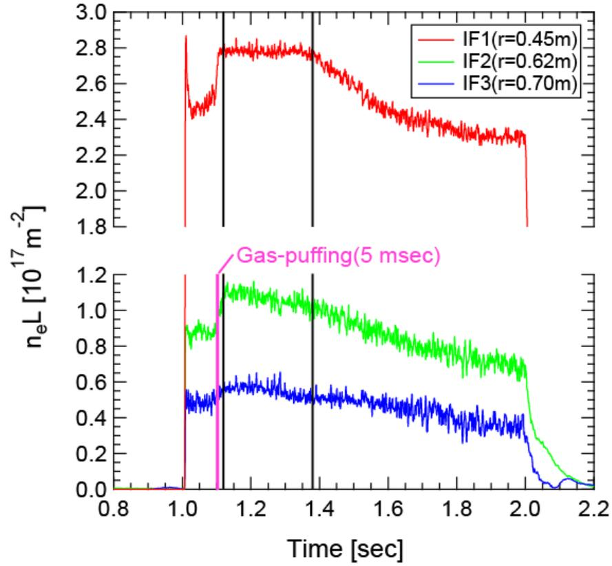
FIG. 3. Time evolution of the line-integrated densities where the chords of the interferometers pass through the inner and the outer edge regions ( $r = 0.45, 0.62, \text{ and } 0.7 \text{ m}$  are the innermost radii of the chords). The innermost chord IF1 observed the constant electron density from  $t = 1.12$  to  $1.38 \text{ sec}$  (black lines), while the other chords decrease.
