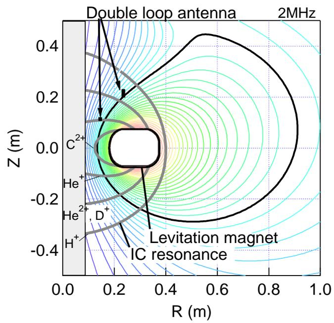
FIG. 5. ICRF antenna and ion cyclotron resonance layer in the RT-1.
