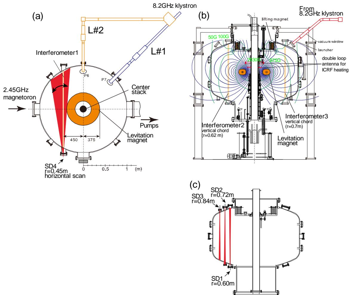
Fig. 1. (a) Midplane from the top. (b) and (c) cross sectional views of RT-1. The line of sights for interferometers are indicated. SD1, SD2, and SD3 indicate the vertical chords for x-ray detectors. SD4 scans horizontally on the midplane.
