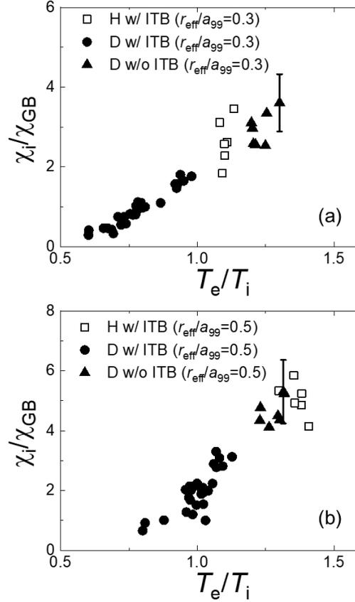
FIG. 3. The heat diffusivity normalized with gyroBohm factor as a function of temperature ratio at (a)  $r_{eff}/a_{99}=0.3$  and (b) 0.5. The typical uncertainty in estimation of heat diffusivity is also shown, which is mainly caused by evaluation of temperature gradient with transform from major radius to averaged minor radius and heating power calculations.
