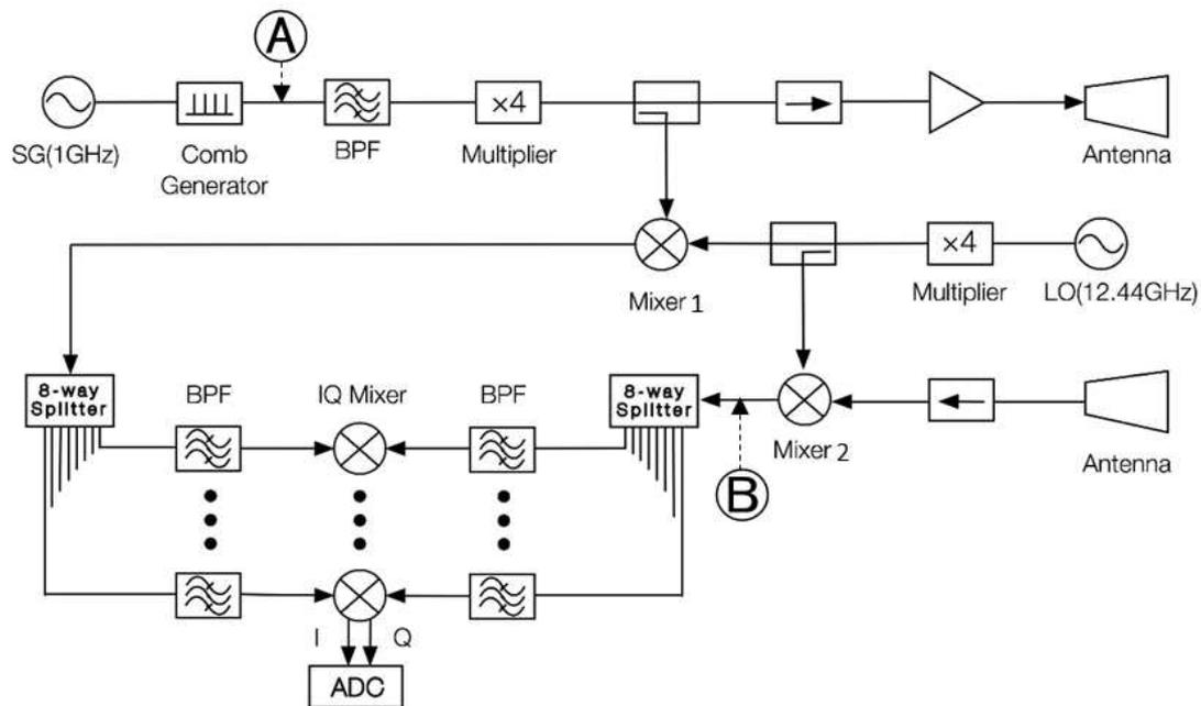
Figure 1. Schematic drawing of U-band microwave reflectometer circuit consisting of a comb generator.
