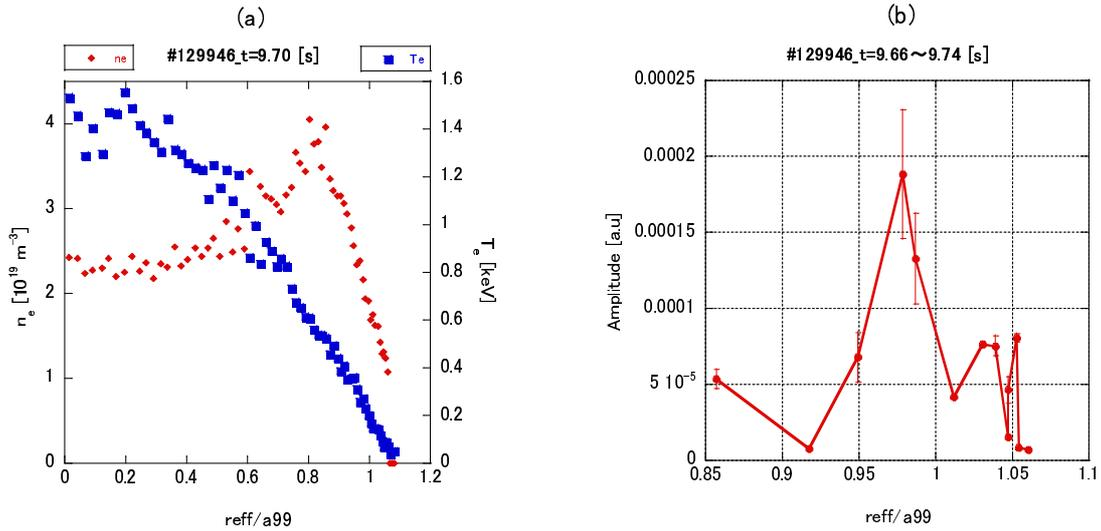
Figure 7. Radial profiles of (a) electron density ( $n_e$ ) and temperature ( $T_e$ ) measured by Thomson scattering system, and (b) the density fluctuation amplitude caused by low- $n$  interchange mode instability.
