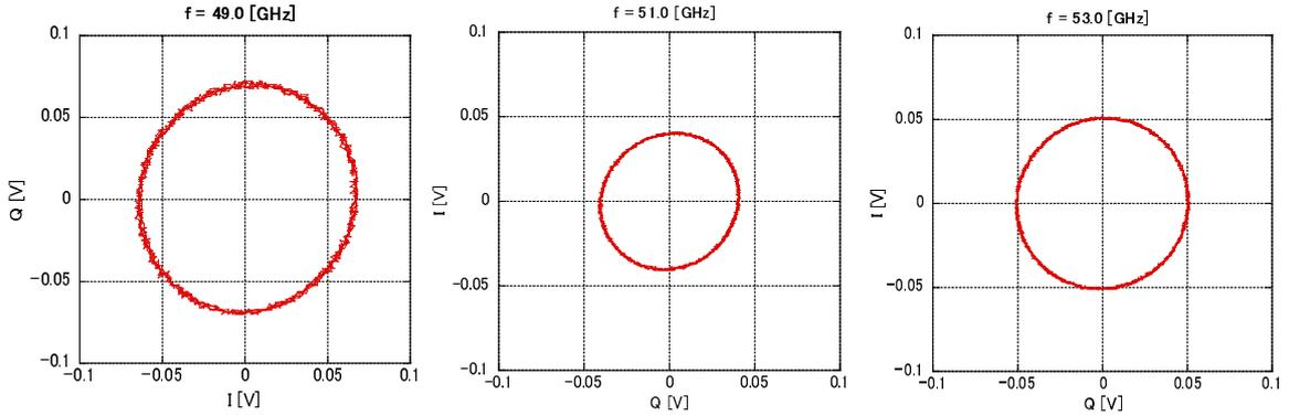
Figure 4. Example of the phasor plot (IQ-plot) of 49.0, 51.0 and 53.0 GHz frequency component
