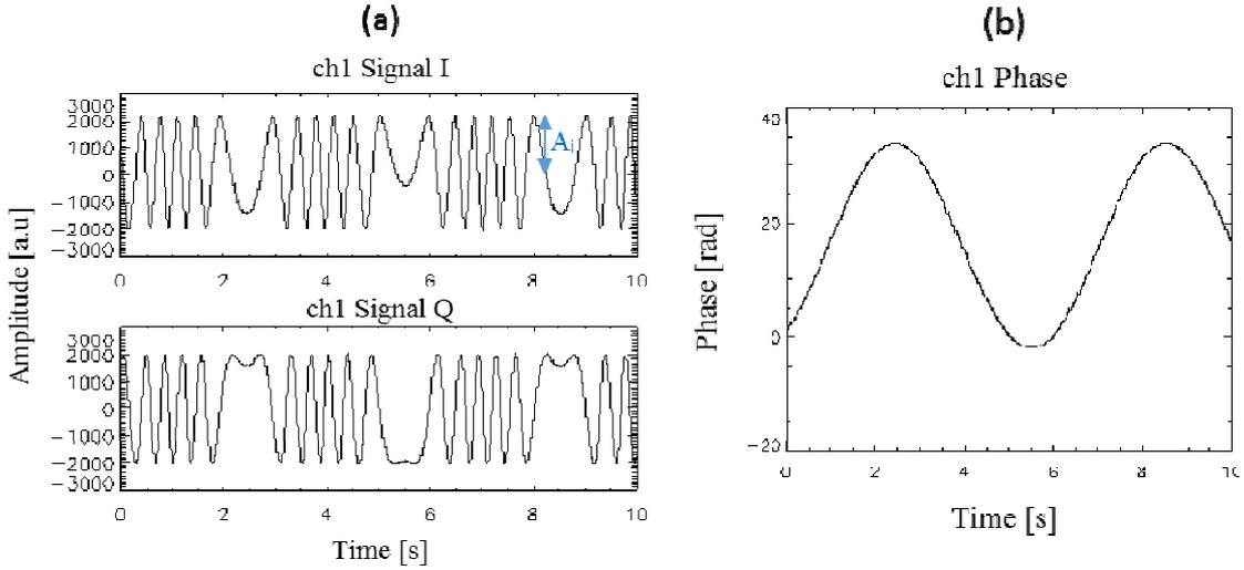
Figure 5. (a) Example of temporal behavior of signal I and signal Q of ch1 (49.0 GHz) and (b) the corresponding phase change in the in situ calibration test.
