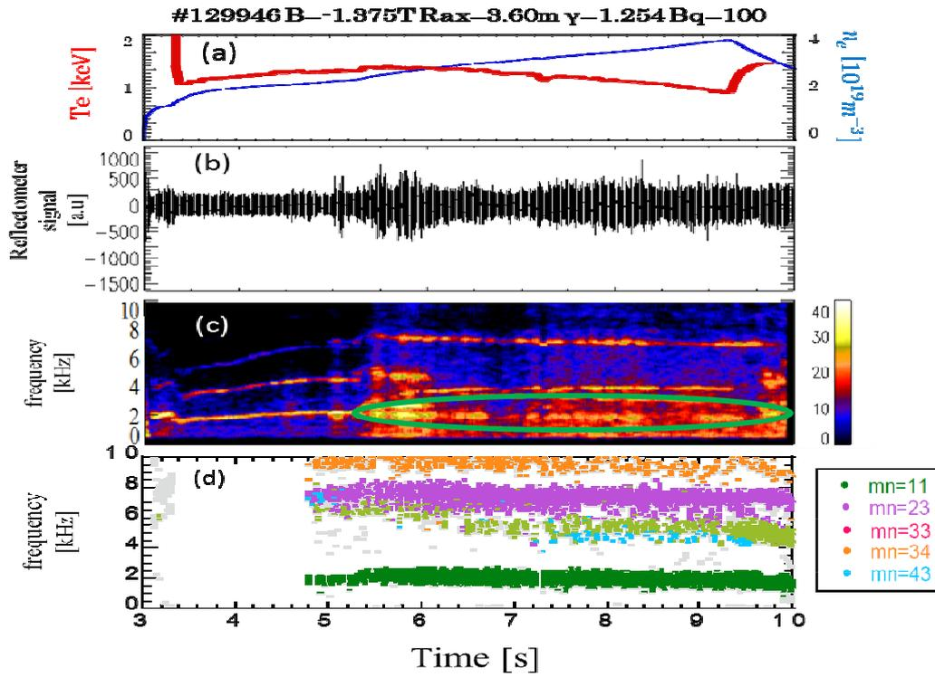
Figure 6. Temporal behavior of (a) the electron temperature ( $T_e$ ) measured by Thomson scattering system [10] and the line-averaged electron density ( $n_e$ ) measured by FIR interferometer [11], (b) 53.0 GHz reflectometer signal, and (c) its frequency spectrogram, and (d) magnetic fluctuation decompositions for the mode  $(m,n)=(1,1), (2,3), (3,3), (3,4),$  and  $(4,3)$  evaluated by magnetic probes signals.
