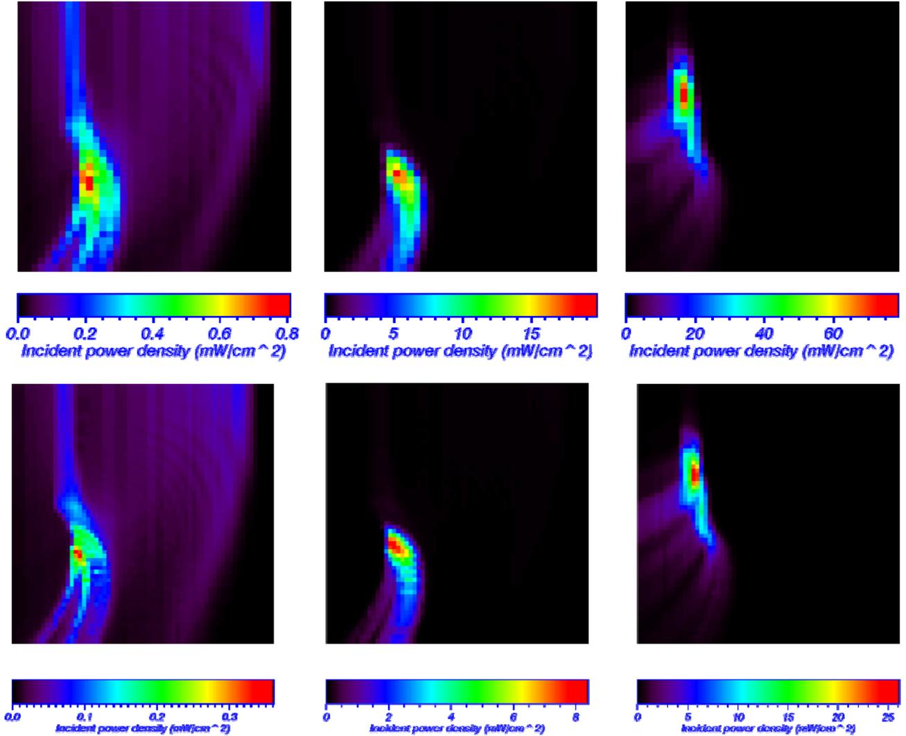
FIG. 3. Synthetic images for carbon and deuterium radiation from SOLPS data for the  $\mu$ bolo (upper row,  $N_{bol} = 40 \times 40$ ) and InSb (lower row,  $N_{bol} = 64 \times 64$ ) cases for core densities of 2 (left), 5 (center) and 10 (right)  $\times 10^{19}/\text{m}^3$ .
