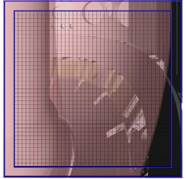
FIG. 2. CAD of FoV of IRVB with tangential view of NSTX-U for  $\mu\text{bolo}$  case with 40 x 40 channels indicated by the gray grid. The plasma is indicated by pink and the blue border lines indicate the 9 cm x 9 cm edge of the foil and the 8 cm x 8 cm edge of the usable portion of the foil.
